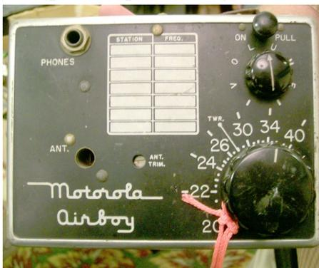
The Motorola Airboy: An example of an LF receiver used by aviators.
