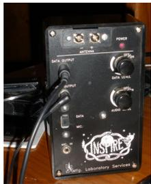
The INSPIRE receiver is designed to amplify the signal in the audio range. There have been improvements in the design, and I understand the new version, VLF-3, has a better filter to
