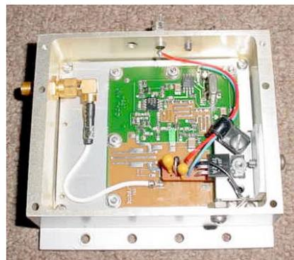
**Photo E - Remounted PLL with Voltage Regulator**
