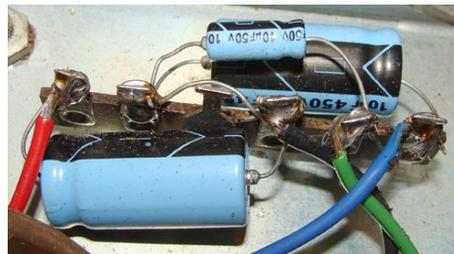
Fig. 4. The three-capacitor assembly replacing the original multisection electrolytic.
