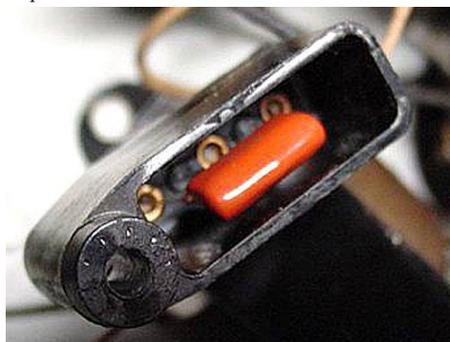
**Fig. 2.** With the potted capacitor removed, a modern unit can be installed in the Bakelite block. Gary Maker photo.
