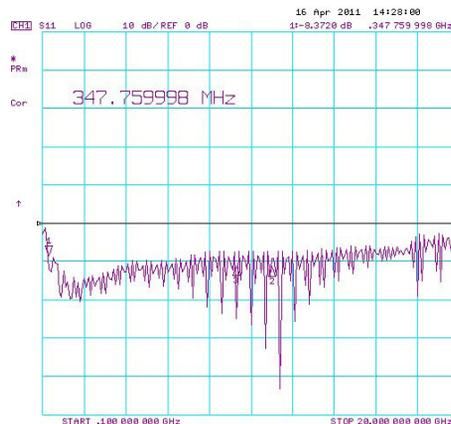
I show the sweep in Plot 1. The 7" Copper disk version was swept in frequency from 100 MHz to 20 GHz. The vertical scale is 10 dB per division. -10 dB Return Loss is equal to about a 2 to 1 SWR. So the 7" disk has a better than 2 to 1 SWR from 350 MHz to 7 GHz and is still working great at 10 GHz. Now you see what I mean when I say these antennas really don't have an upper frequency limit.
