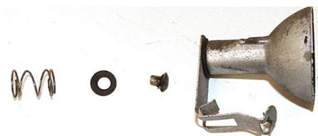
*Pilot light fixture ready for reassembly.*
