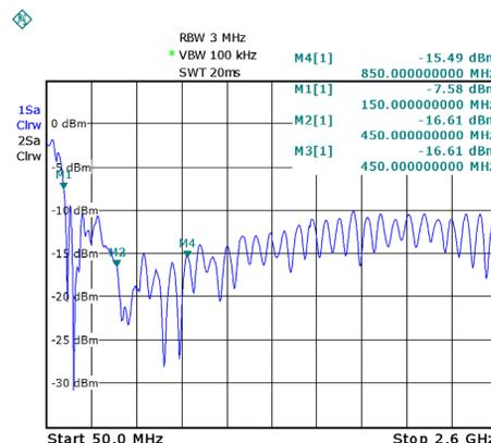
In Plot 2 I show a sweep with a better view of the low end of the frequency range of the larger planar disk antenna, this time on my analyzer. Again -10 dB return loss is equal to about a 2 to 1 SWR. So we have a 2 to 1 or better SWR from just over 150 MHz to 2.6 GHz and beyond.
