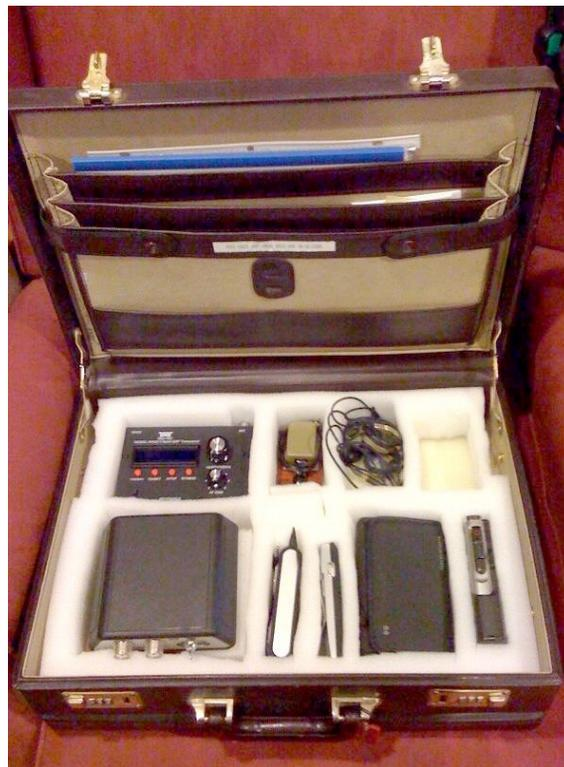
The center insert holds the radio and accessories that you wish to carry. Once these items are placed where you want them they are traced onto the foam and these tracings are cut out to hold the equipment. The nice thing about not gluing the bottom and center foam together is that the center insert can be easily replaced with another insert that is cut for different equipment allowing you to configure gear for your travel and operating needs.
