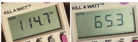
*As shown on the P3 KILL A WATT, when powering a 500-W load, Old Betsy is putting out 114.7 V at 65.3 Hz — a bit out of spec after 14 years! I guess it's time to find a service manual and adjust the governor and the AVR controller.—NT0Z*
