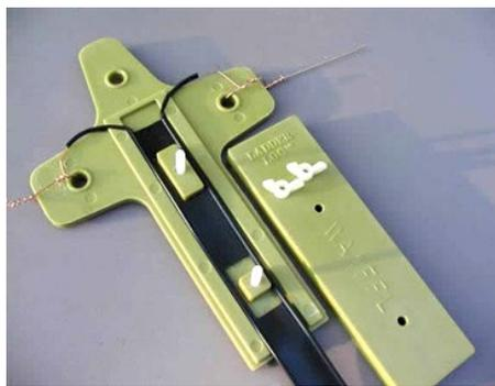
Use this WA1FFL Ladder-Loc center feed connector (\$13) if you use ladder line and no balun. (Courtesy: Universal Radio)
