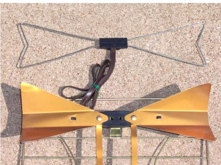
been made out of sheet Aluminum to form a wide and broadband element. Above it is where the wire has been formed into a "bowtie" shape to again make the equivalent of a fat dipole. The bowtie is not quite as wide in frequency as a fat dipole or the sheet metal version, but it's pretty close and the bent wire is a lot cheaper to make.
