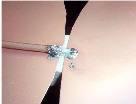
In Photo D you can see how the coax is attached. You want the leads VERY short for best high frequency response. I find that the Teflon insulated coax is the easiest to work with, but RG58 can be used if you solder very quickly.
