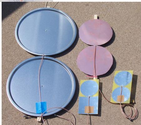
This month I have an extremely broad band antenna design that makes a great scanner antenna. This family of antennas goes under a variety of names: Planar Notch, Elliptical Dipole, Planar Disk or Planar Circle dipole. These antennas were first described by Walter Stohr in the 1960s and they are noted for their extremely wide bandwidths.
