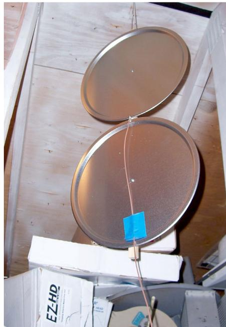
As you can see in Photo E, I just drilled a hole in the top of the wood support, a bit of thin rope, and hung the antenna from a rafter in the attic.
