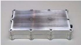
The [WR-G33RSS Signal Strength Measurement Module](#) is a specialized OEM building block suitable for a variety of industrial, scientific and other specialist applications where the ability to measure received signal strength within LF, HF, VHF and UHF frequency range is required.
