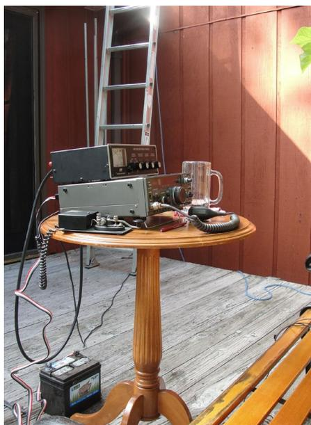
*Field Day 2011 station set-up: HF transceiver with antenna tuner feeding 10 watts into a 20 foot extension ladder leaning up against the wall. Power is provided by a lawn tractor battery. (Courtesy: Author)*
