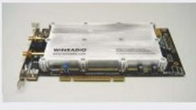
The [WR-G39WSBi Sonobuoy Telemetry Receiver](#) is a low-cost, high-performance internal PCI-card-based receiver primarily designed to receive sonobuoy signals in military or civilian marine telemetry applications.
