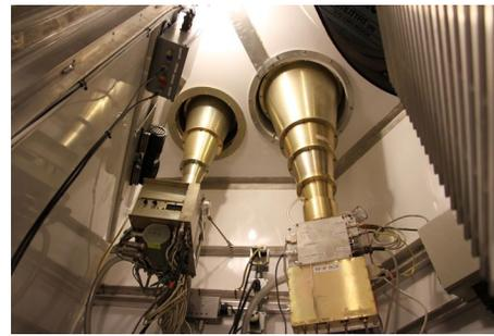
Above is a view of a couple of the horns. Note one of the boxes is labeled 'RF/IF BOX'. At this point, the IF (Intermediate Frequency) is converted to digital signals and sent on into a shielded room near the control room where the 'correlator' or computer processing system handles the incoming data for all of the dishes simultaneously. The data is sent to the VLA's center in Socorro, NM some 50 miles away via fiber optics.
