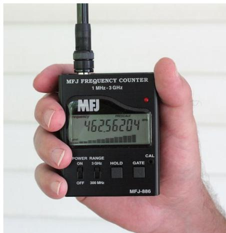
The MFJ-886 in action, showing the 10 digit frequency display and the LCD bargraph at full deflection.
