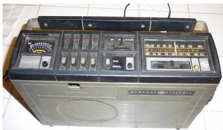
General Electric made just such a radio that is a nostalgic favorite of mine. Called *The Searcher*, this mid-1970's era portable radio offers coverage for the commercial AM and FM bands as well as four channels covering the VHF (Very High Frequency) Hi Band, noted on the radio itself as the Public Service Band (PSB). Each channel can tune independently between 150 MHz and 174 MHz via four tuning knobs located under a protective cover.
