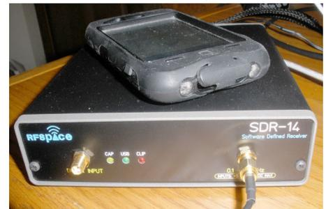
On the front panel, the yellow *CAP* light tells you're actively gathering data. The green *USB* light is lit when you are connected to the PC running software SDR-14 aware. The *CLP* (clipping) light comes on when you are over-driving the unit. You can set the preamp-gain to a more negative setting to reduce the gain. I used the -10 dB setting.
