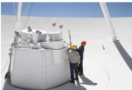
Above is the entry point to the horn antennas/detectors. Notice that the cluster of horns are offset, aimed upwards toward the secondary reflector above. Each horn is designed for operating on different bands. The little lamps are heat elements to dispel ice and frost and even rain drops. It has been known to happen even out in the desert. We climbed up a ladder onto the surface of the dish through a trap door near the ladder.
