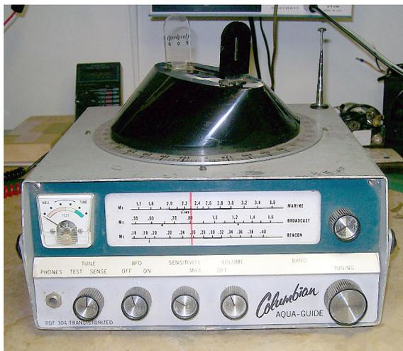
To test the unit's speaker, I disconnected it from the circuit and temporarily connected a "test" speaker with alligator clips. I was hoping for quick success, but the substitute speaker made no real difference in audio quality. I tuned in several strong signals across the AM broadcast band, and all were low and not very clear.
