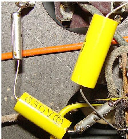
Close shot of replacement capacitor shows use of butt connectors in making the changeover.
