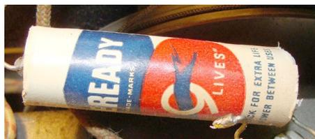
*Ancient Eveready penlight cell had been soldered in to replace a dried-out Mallory bias cell. As it still provided 1.5 volts on the nose, I left it in place.*
