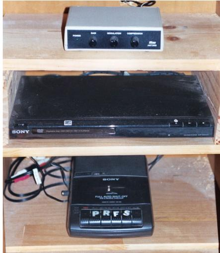
*The author’s personal broadcasting facility consisting of a low-power, limited-range AM transmitter plus a CD/MP3 player and a cassette tape player. From here, recordings of Golden Age radio material from the author’s personal collection can be broadcast to an assortment of vintage tube radios scattered around his house.*
