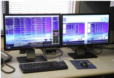
The dish operator monitors the various parameters displayed on the screens above. Note the DC power supply behind the Dell monitors. The monitors are run by highly regulated and filtered DC (direct current) power supplies in order to minimize RF (Radio Frequency) noise often associated with switching power supplies built into standard monitors.
