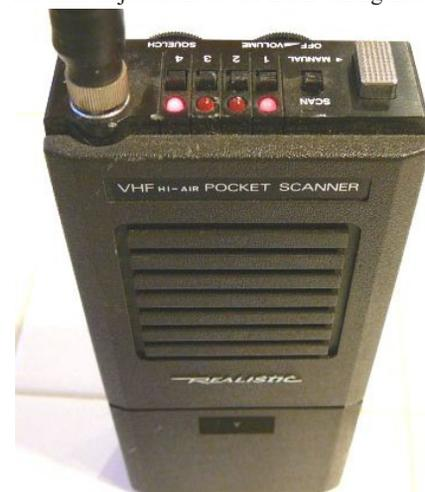
Crystal-based scanners could continuously check multiple frequencies, but the expense and mechanical effort necessary to add new frequencies put a limit on the dynamic flexibility of these units. Physical size and circuit board layout constraints also limited the number of crystals that could be accommodated, so there was an upper boundary on the total number of frequencies a scanner could support.
