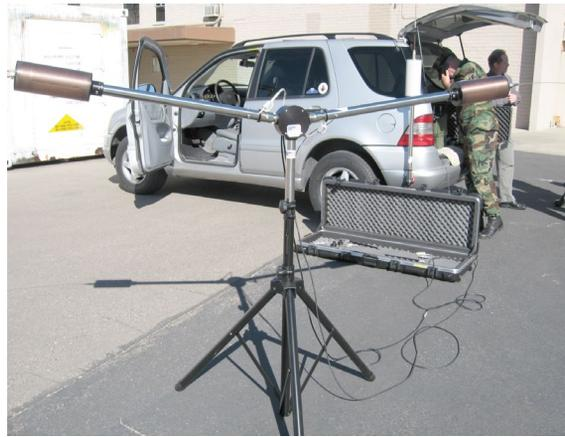
*Hi-Q Military portable HF NVIS antenna (Courtesy: [www.hi-qmilitaryantennas.com](http://www.hi-qmilitaryantennas.com))*
