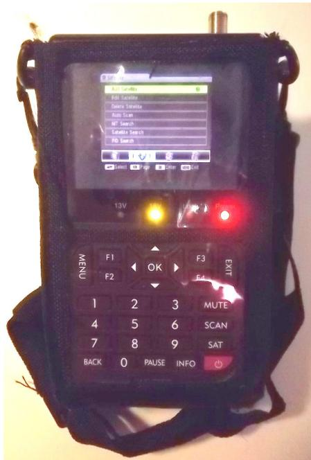
*Satlink WS-6906, in the “On” position, with Power and 18V LEDs on. LCD display can be turned on and off using F1 key. Case and strap are useful when using outdoors to prevent scratching, and strap is used to hang unit around neck and prop against chest for easier viewing. Note that the carry case top flap can be folded over for easier viewing in bright light.*
