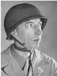
**Fig. 5.** Here, reduction of external noise is accomplished by fastening two carbon mic units to a strap fastened tightly high on the user's neck. Reproduction of this throat mic was less than perfect, lacking high frequencies.
