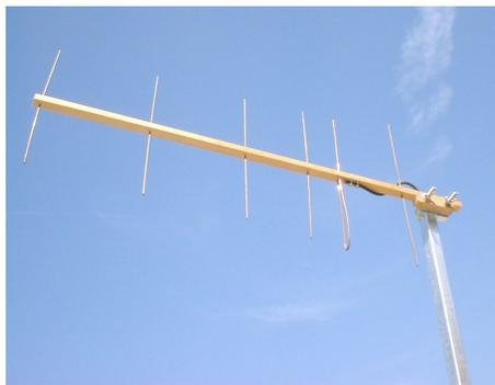
**Photo E - 460 MHz Beam antenna**
