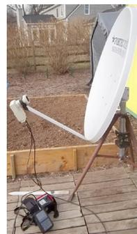
*Fortec 90cm Ku dish, Invacom Quad Polar Legacy LNB mounted on tripod with leveling device on mast. Attached to the LNB are the WS-6906 and Channel Master Model CM-1007A Signal Level Meter. Just above the meters is a white picket that has a compass glued to it pointing to magnetic South. I could not remove neighbor's house from picture, hi hi.*
