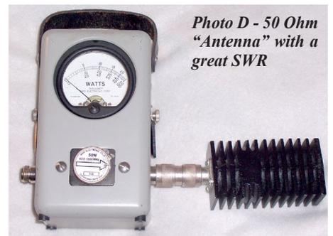
Photo D - 50 Ohm "Antenna" with a great SWR
