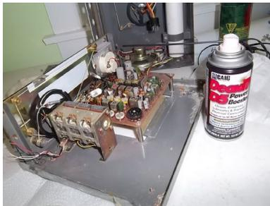
**Coastal Navigator chassis cleaned and ready for checkout.**
