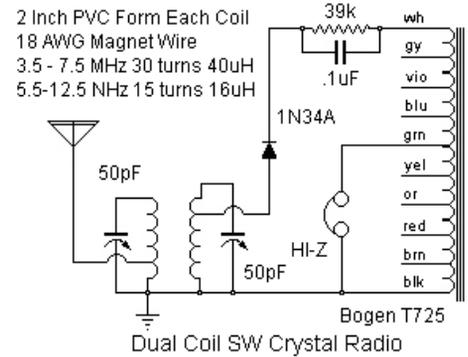
**The MT Special Dual Coil Shortwave Crystal Set Schematic.**
