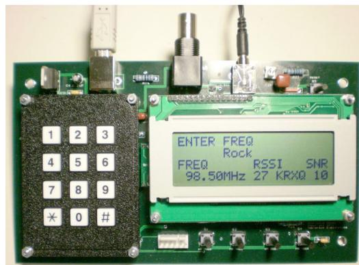
The Shortwave Daddy is built around a professionally-laid-out PC board utilizing high quality components. All factory pre-drilled holes are “through hole” making soldering a more reliable process. The few connections for surface-mount connections, and the surface-mount parts themselves, are solder-plated for more secure attachment.
