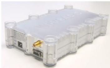
**WiNRADiO G305E (\$900) offers 9 kHz to 1800 MHz coverage in a PC-based receiver. (Courtesy: Grove Enterprises)**
