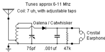
Remove resistor for magnetic earphone.
