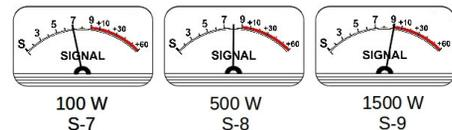
*S-meters showing how power at 100, 500 and 1,500 watts is heard. When measured on the other op’s S-meter, the rather minimal signal boost provided by RF power amplifiers is starkly apparent. (Courtesy: Author)*
