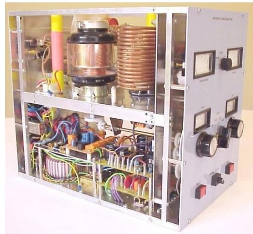
*RF power amplifiers can be a "rite of passage" for advanced home-brewers, and some, like this 160-10m "desktop kilowatt," designed, built and tested by Mark Marsden, G4AXX, over a four-year period, are real works of art. Built around an Eimac 4CX1000A triode, the amp runs on 230 V AC and puts out 1400 W PEP from 25 or 100 W of drive (selectable). See more at [www.granta.g4axx.com/linear.php3](http://www.granta.g4axx.com/linear.php3). (Courtesy: Mark Marsden G4AXX.)*
