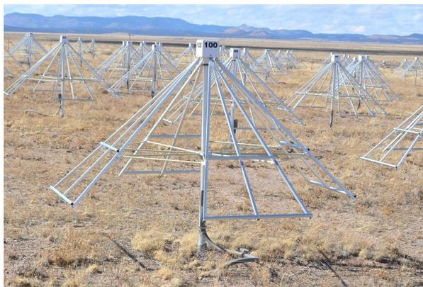
Note that the antenna elements are somewhat aligned with an east-west and north-south orientation. The antennas are not in perfect lines due to phasing of the pattern requirements. There is a coax cable run from each antenna into a small building. Each cable is lightning protected.
