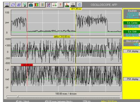
Figure 2: MFA Pyongyang FSK ARQ Signal Timing
