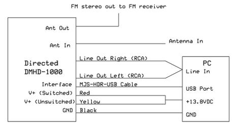
The antenna output is not a pass-through antenna to be used when the unit is off. There's actually an FM modulator inside so that the decoded stereo can be fed into a car's FM radio antenna input. When used with a PC in the application being discussed here, you must use the line out audio jacks.
