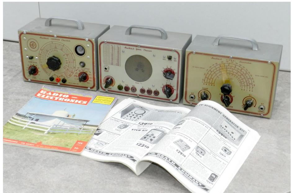
G-1, C-1 and T-2 make up the Heath 1948-49 test bench.
