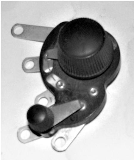
*Accessory input switcher slips over antenna binding posts, allows rapid switch selection of any of the six possible antenna configurations.*
