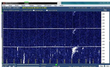
If you're new to the FUNcube concept, the receiver provides up to 96 KHz of bandwidth to one of several programs such as SpectraVue. It can demodulate the signals and the audio can then be fed to a variety of programs such as the ARGO chart shown above.
