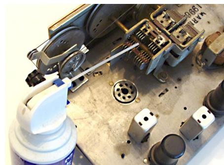
*A compressed air spray can is very useful for cleaning between variable capacitor plates.*
