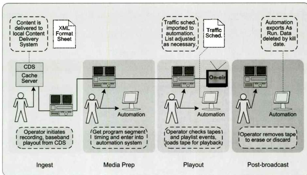
Figure 2. Manual Content Delivery Process and Workflow Tasks
