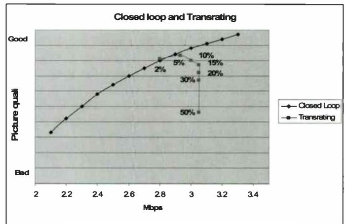
The blue curve represents the picture quality of the closed-loop system, where the quality steadily improves as the average bit rate is increased from 2.1 to 3.3 Mbps. The pink curve is the quality measured on the transrated content where the average bit rate reductions required changes from 2% to 50%.
