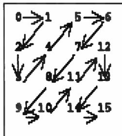
Figure 7. Scan pattern for a transformed 4x4 block for frame coding in H.264
