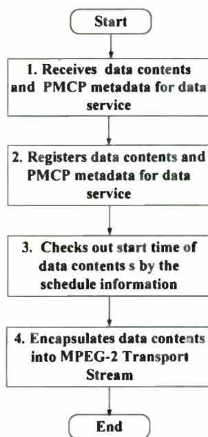
Figure – 9. The operation flow of data server
