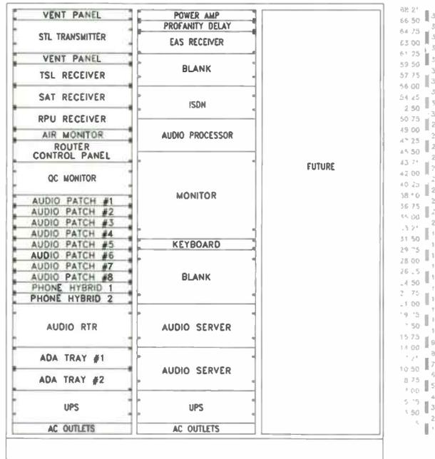
FIGURE 2: Rack Elevation Drawing
