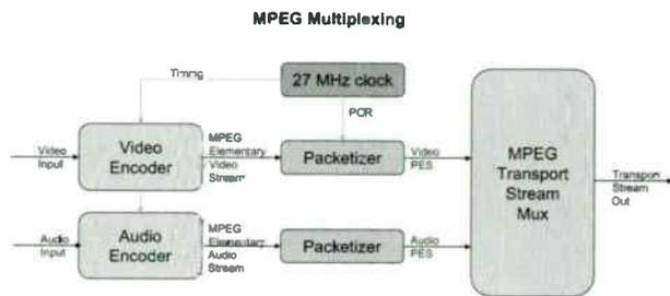
This stamping and synchronization allows streams to be placed into transport stream wrappers so that they can be sent across a network and reassembled in order at the receiving end.
