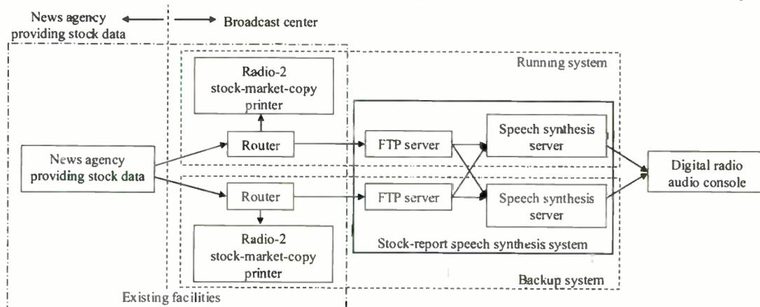
Figure 7. Stock speech synthesis system for digital terrestrial radio
