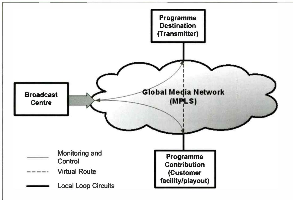
The original distribution network connecting our UK transmission sites was based upon a hybrid of satellite and ATM platforms. Both had been reliable, but the ATM infrastructure was expensive to operate and was reaching the end of its design life. Our international distribution and contribution was largely satellite based, with some ISDN and private leased circuits. Programming for non-live playout and
