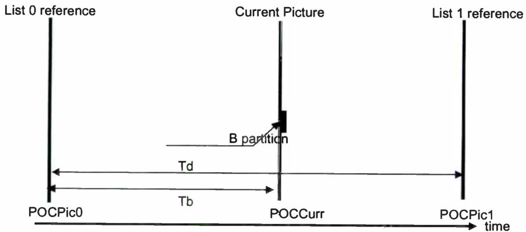
Figure 14. Temporal distance determination
