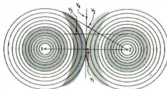
Fig. 5 — Plot Illustrating Doppler Effects in Mobile Receivers for Synchronous Stations 1 & 2
