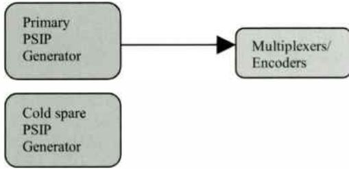
Figure 3. Cold Spare Redundant System
