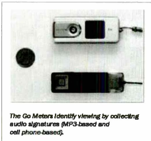
**The Go Meters identify viewing by collecting audio signatures (MP3-based and cell phone-based).**
