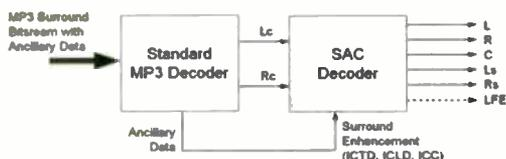
Figure 4: General structure of an MP3 Surround decoder.
