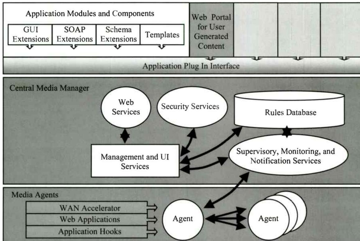
Figure 5 Components of a managed digital media distribution system
