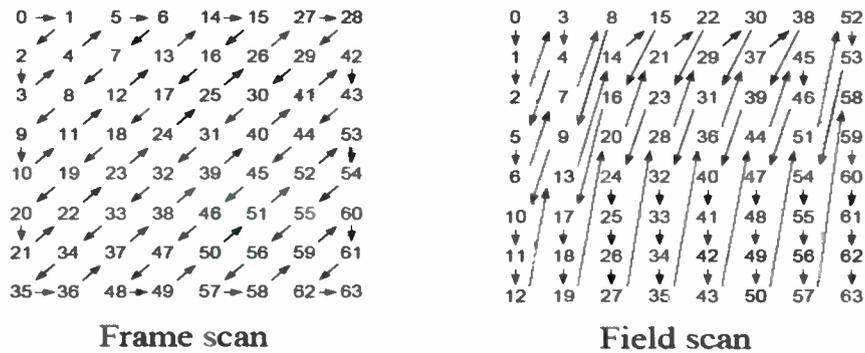
Figure 8. Frame and field Scans for 8x8 blocks in H.264
