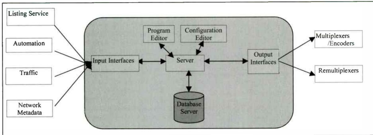
Figure 1. Metadata (PSIP) Generator system
