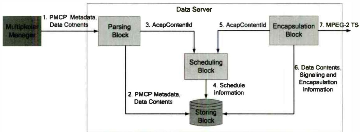
Figure – 8. Data server block structure based on PMCP schema for data service
