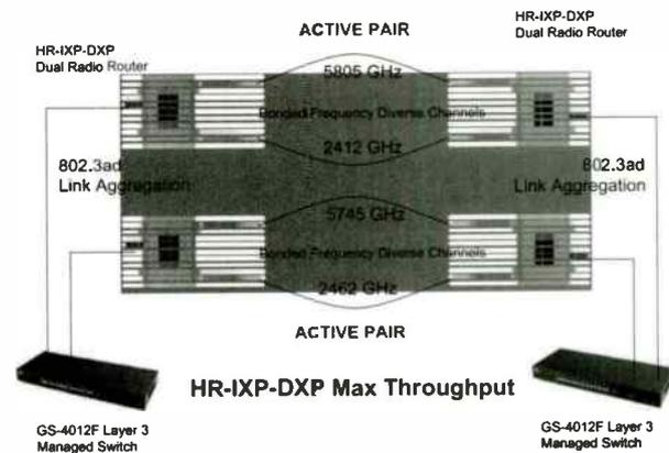
In either method, interfaces are grouped together into logical trucks. The router monitors the condition of each physical interface in the trunk. If the link is up and running, then traffic is forwarded over it and the interface remains active in the trunk. If the link is down, traffic is routed to alternate interfaces and the interface is removed from the trunk.
