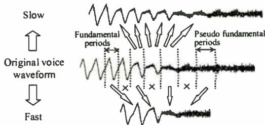
Figure 8. The conceptual figure of speech rate conversion
