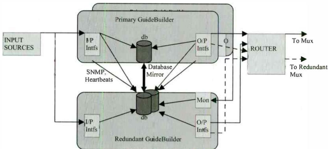
Figure 5. N+M Redundancy configuration
