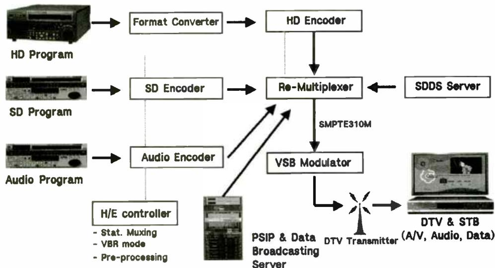
Fig. 2. MMS End-to-end System
