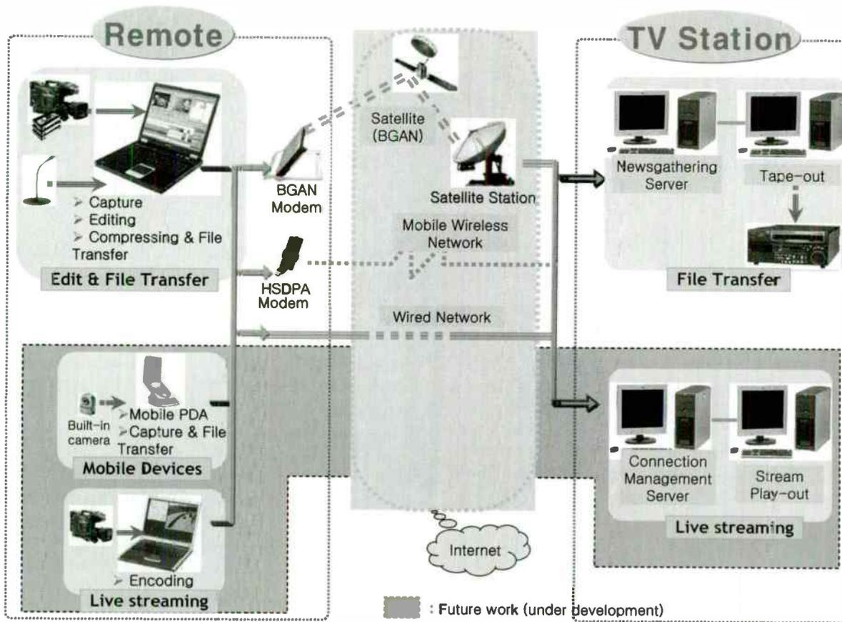
Figure - 1 the workflow of the system
