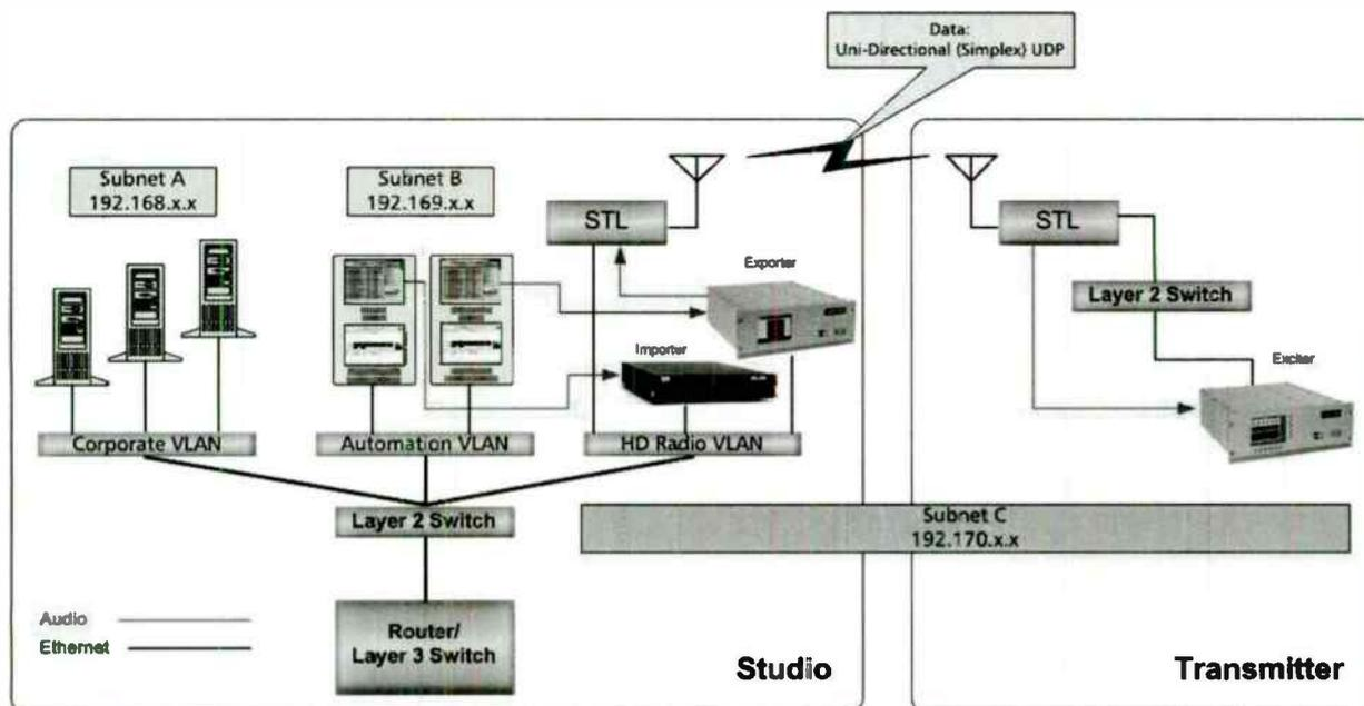
Figure 8: Multicast Network Architecture, HD Generation at Studio Side
