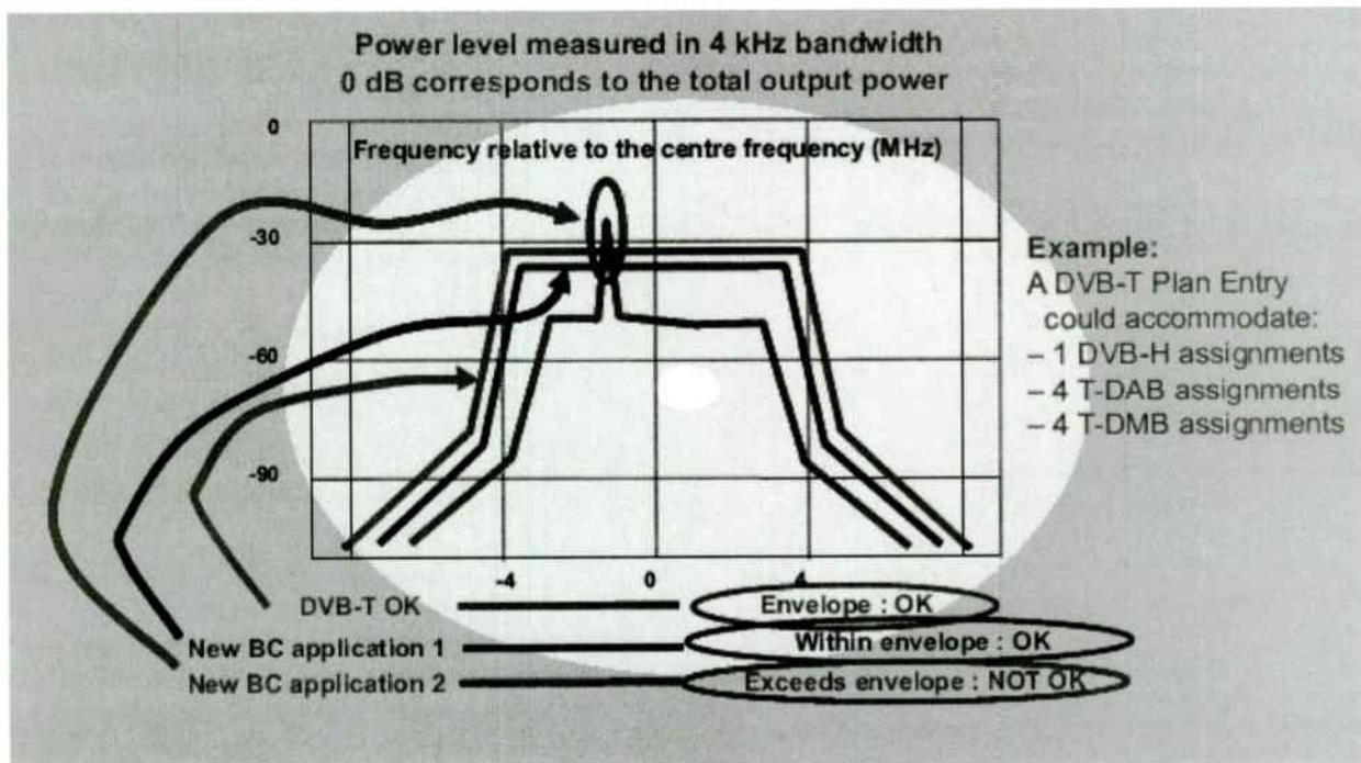
FIGURE 8 – The “envelope” or “mask” concept (Source EBU)
