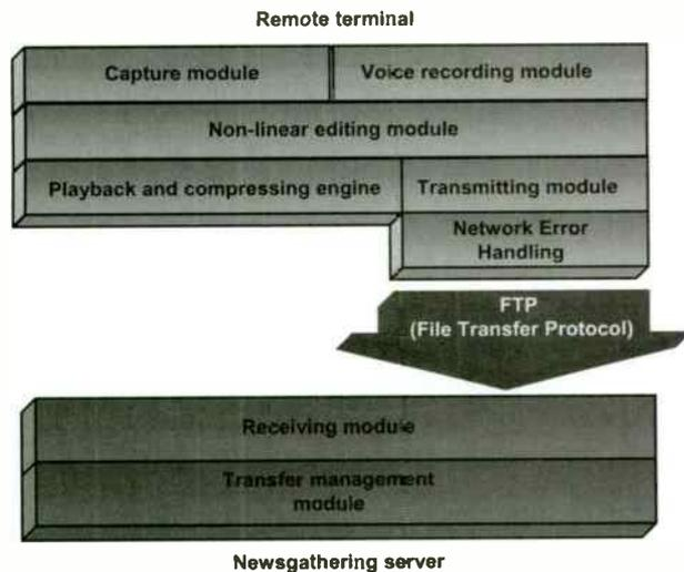
Figure - 2 the system architecture
