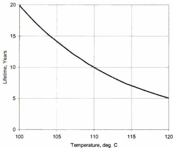
Figure 5: Lifetime reduction and conductor temperature
