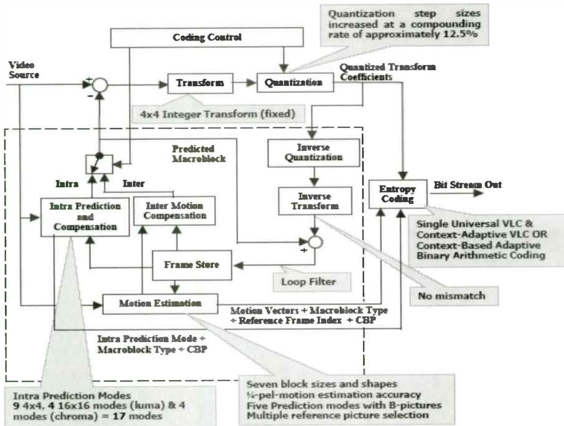
Figure 1. Block Diagram of the H.264 encoder (Original Specification, 2003)
