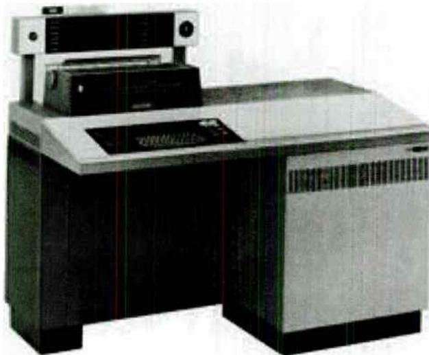
Fig. 1 A basic IBM 1130 CPU with hard drive cabinet.
