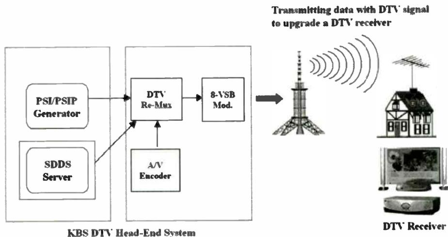
Fig. 4. Concept Diagram for SDDS
