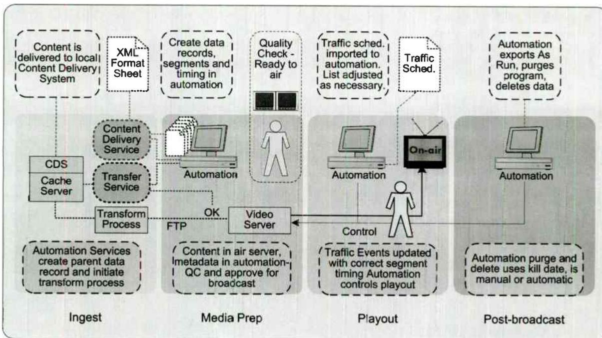
Figure 3. Automated Data-Driven Content Delivery Process and Workflow Tasks
