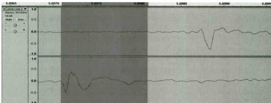
**Figure 3: An isolated impulse in digital (upper trace) and analog (lower trace), with an apparent 71 sample offset (analog lags digital). The shaded area represents 46 samples offset, which was measured by the Belar and Audemat during this capture.**
