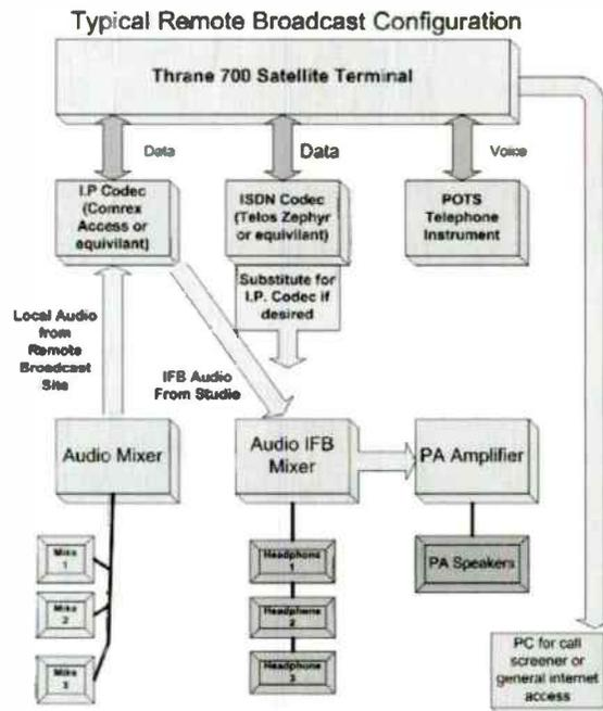
Figure 3. Typical Broadcast Configuration
