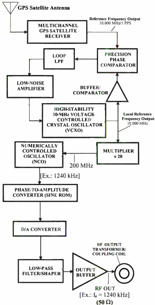
Fig. 2 — Basic GPS-locked DDS Oscillator System
