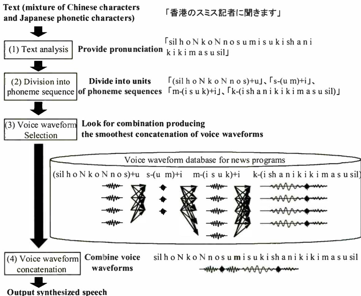
Figure 2. Operation procedure of high quality speech synthesis system
