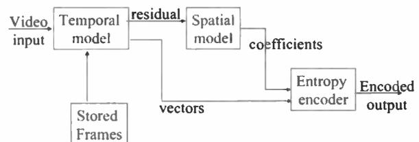
MPEG 4 encodes streaming content using a combination of vectoring and spatial modeling. The input signal is processed by the encoder comparing time sampled image frames and then calculating the differences between frames.
