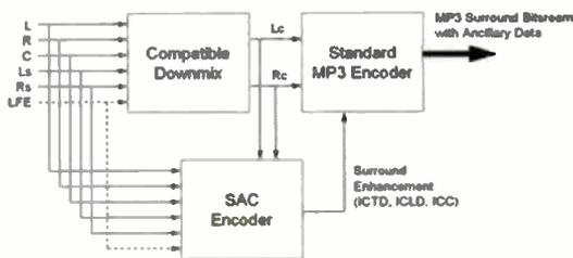
Figure 3: General structure of an MP3 Surround encoder.
