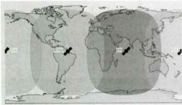
Figure 1. Inmarsat Coverage footprint
