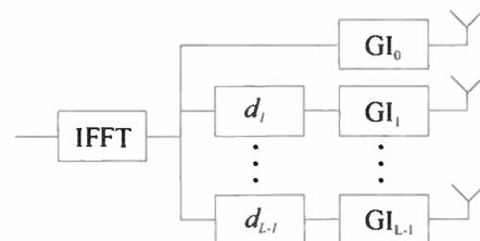
Figure 4. OFDM transmitter with CDD
