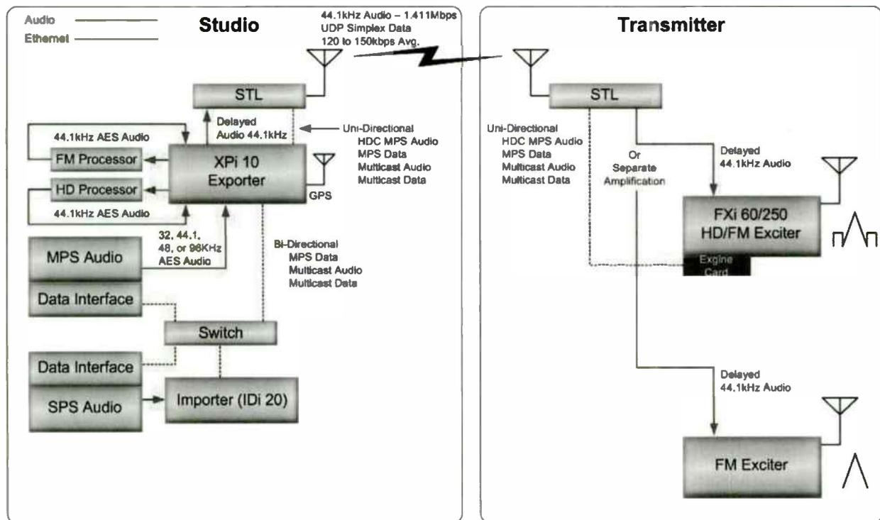
Figure 6: Multicast Architecture, HD Generation at Studio Site
