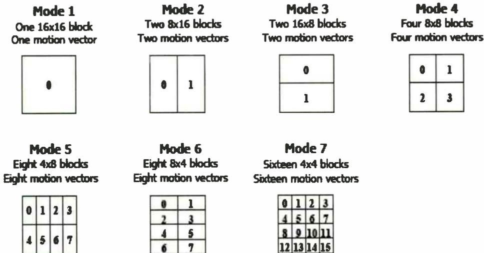
Figure 3. Dividing a macroblock for motion estimation and compensation
