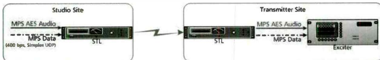
Figure 1: Basic HD STL Configuration. No Multicast
