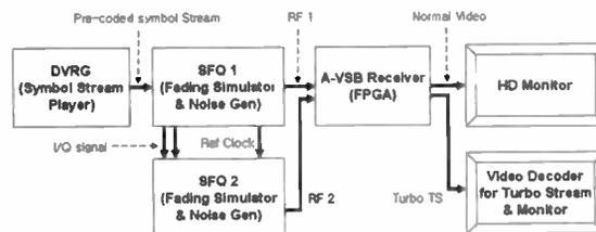
Figure 11 Test Bed for A-VSB System Evaluation
