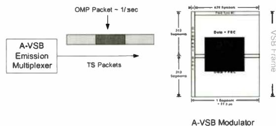
Figure 2 Deterministic Framing between A-VSB Emission Multiplexer and Modulator
