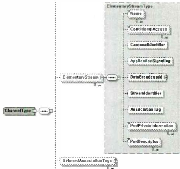
Figure – 5. ChannelType diagram for ACAP data service
