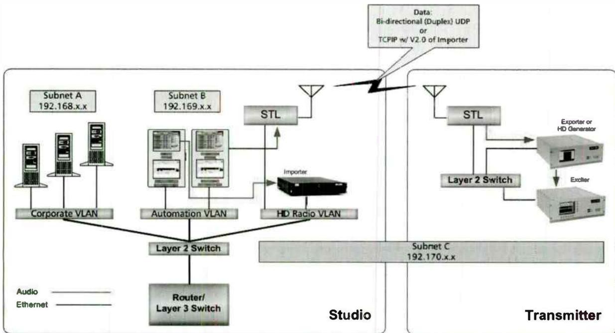
Figure 5: Networking Configuration, HD Generation at TX Site
