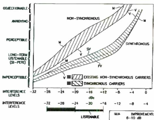
Fig. 4 — Audibility of Synchronous vs. Non-Synchronous Interference
