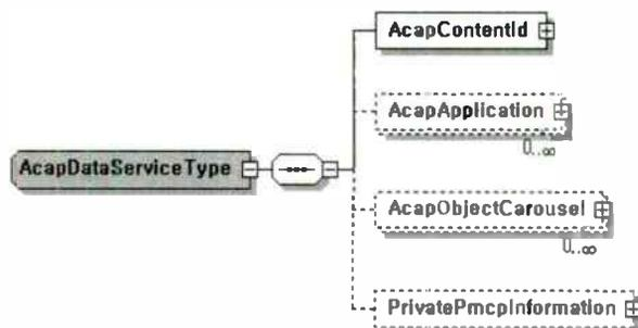
Figure - 6. AcapDataServiceType diagram for ACAP encapsulation and AIT signaling
