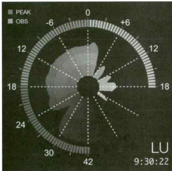
Fig 7. Loudness meter with loudness history in the "radar view" and color coded in accordance with the HDTV targets of Fig 2. The loudness history aspect is not addressed in the BS.1771 draft meter, but an example with such virtues is shown in Fig 7-8. The loudness history can be set at, for instance, one revolution per minute.
