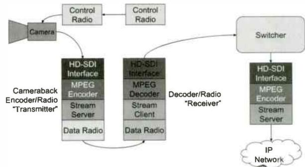
At first glance they appear to provide raw HD-SDI to HD-SDI pipes. But on closer inspection, they use compression encoding in order to fit the video stream into their available bandwidth, then they decompress at the other end. While they may get fairly good results with their compression methods, any signal carried over these solutions, which is intended for rebroadcast (and therefore recompression again) will suffer from cumulative resolution loss due to transcoding.
