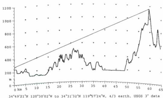
Figure 10. Vandenberg uplink to Broadcast Peak terrain profile. Path is 59.7 km at 123°T. Profile extends 5 km past the ENG-RO site.
