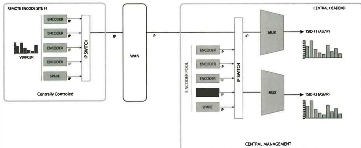
Figure 4 Distributed Encoding Architecture
