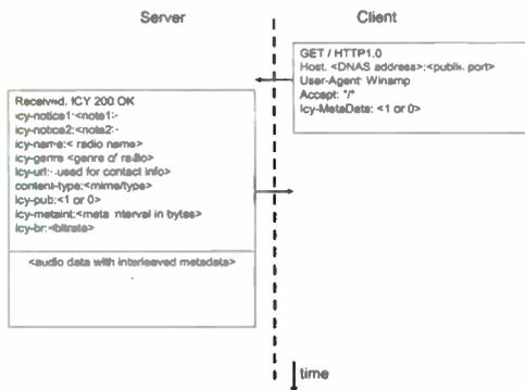
Figure 9: Shoutcast protocol between server and client.
