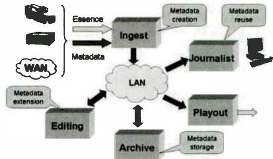
Figure - 3: Structure of a networked studio
