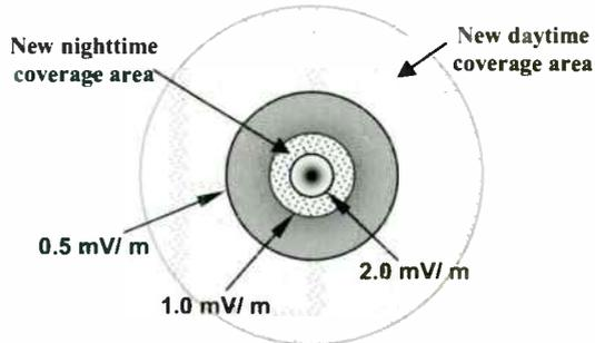
**Fig. 6 — Effective Synchronous Day/Night Interference-Limited Coverage Improvements**
