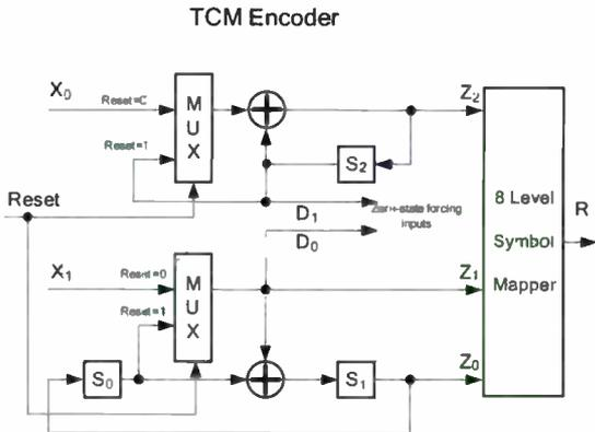
Figure 3 TCM Encoder with Deterministic Trellis Reset
