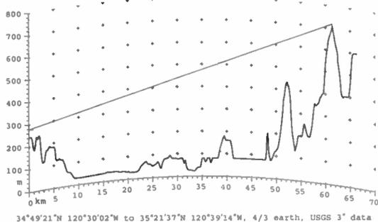
Figure 11. Vandenberg uplink to Cuesta Peak terrain profile. Path is 61.3 km bearing 347°T. Profile extends 5 km past the ENG-RO site.
