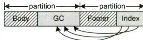
Figure 3: a self-contained partition with backward indexing for VBE essence
