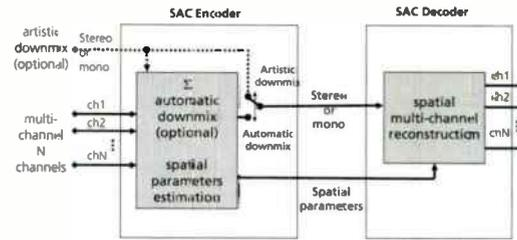
Figure 2: Principle of Spatial Audio Coding
