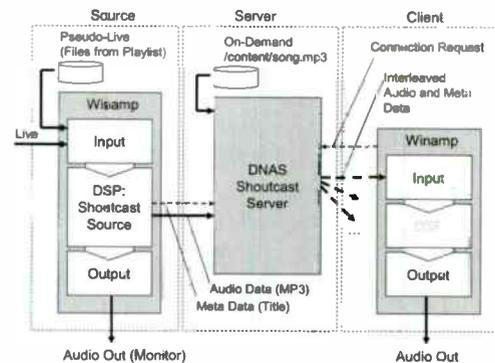
Figure 7: The three components of an Internet Radio system based on Shoutcast: Source, Server, and Client.
