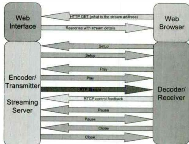
RTP, RTSP and RTCP combined add less than 5% total overhead to any streaming media, and in the case of large files such as an HD stream, they are negligible.
