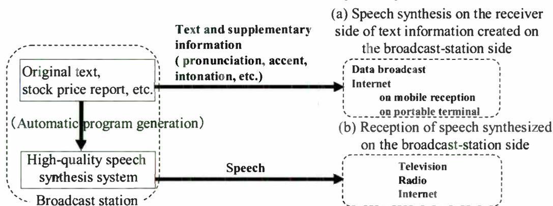
Figure 1. A block diagram of speech synthesis services
