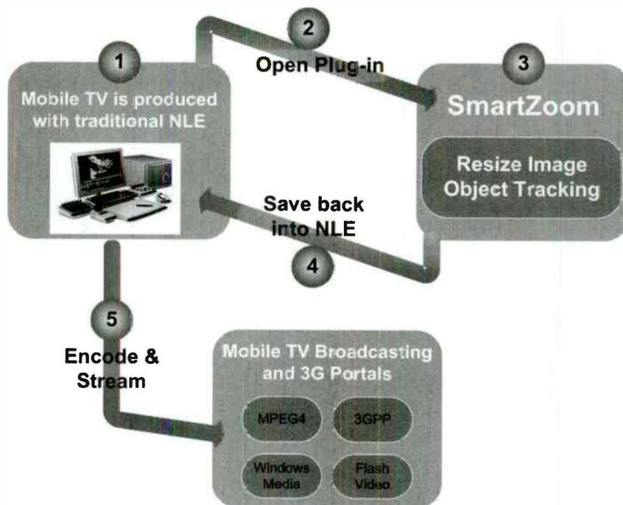
Figure 4: Mobile TV production tool as a NLE plug-in
