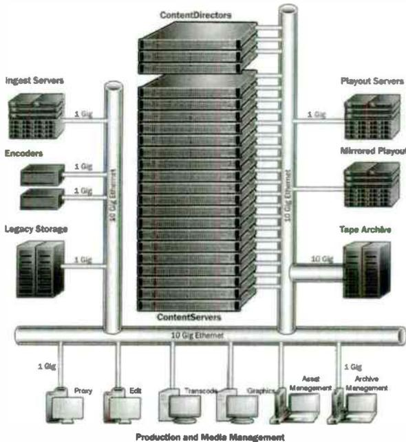
Figure 2. A typical application of media-aware storage (Omneon's MediaGrid)
