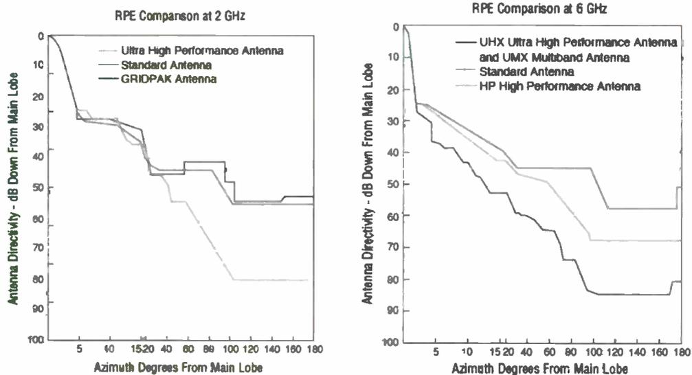
Figures 8 (left) and 9 (right). RPEs for Andrew Corporation standard performance, high performance and ultra high performance parabolic antennas at 2 GHz and at 6 GHz. These figures are courtesy of Andrew Corporation.
