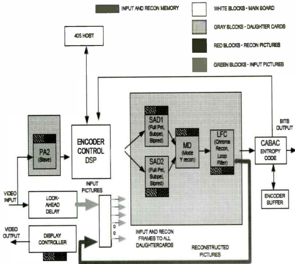
Figure 15. Overview of the SA H.264 SD/HD encoder architecture
