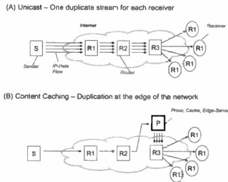
Figure 6: Principle of content caching based on an edge-server compared to unicast.
