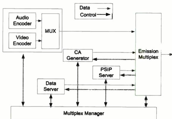
Figure -1. Data broadcast station system
