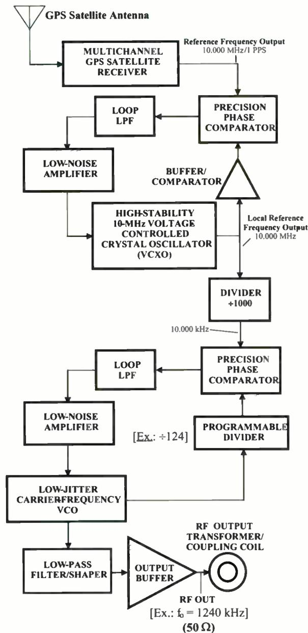
Fig. 1 — Basic GPS-disciplined oscillator system.
