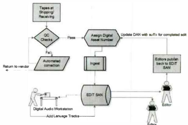
Figure 3. Workflow diagram for a fairly simple editing operation
