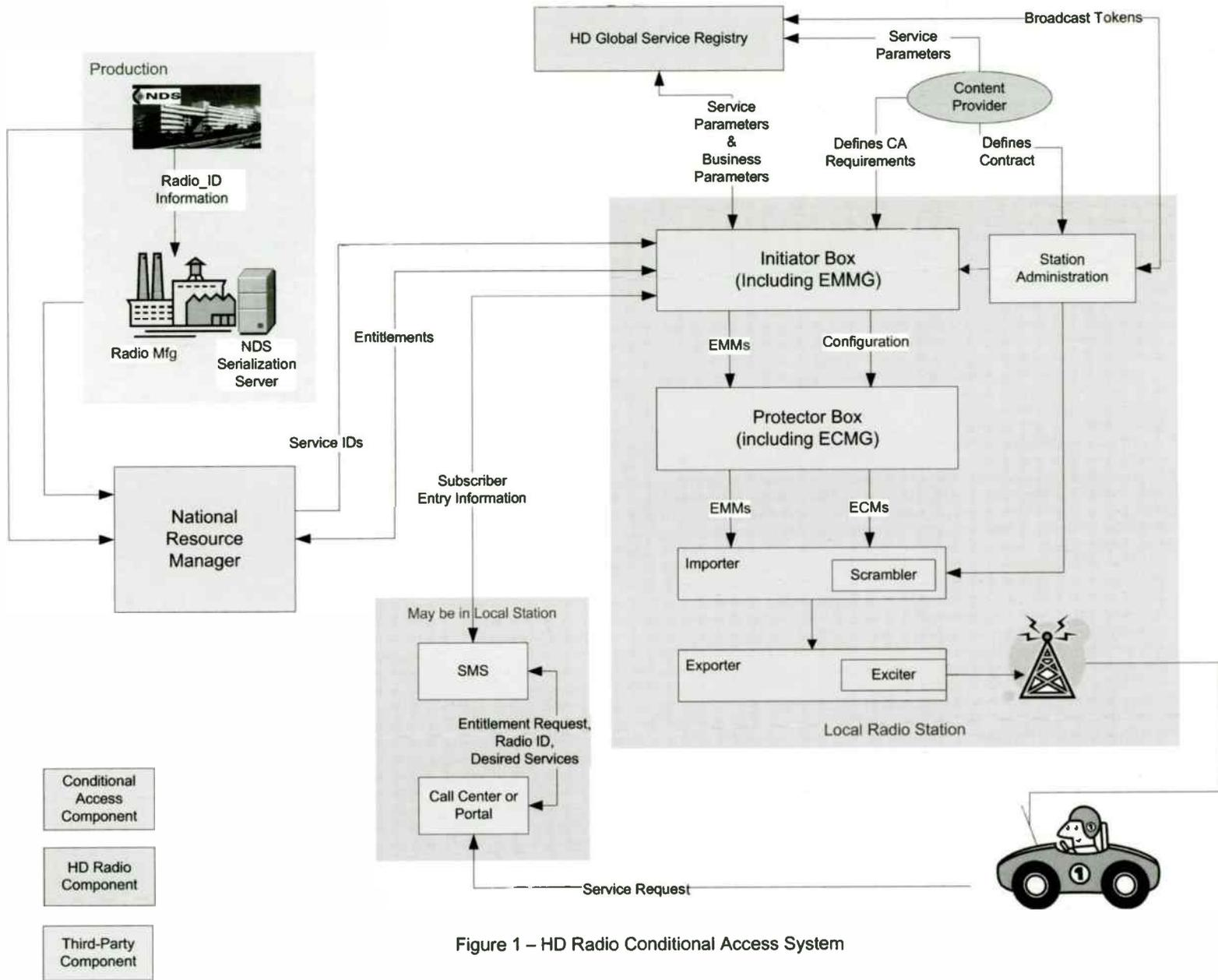
Figure 1 – HD Radio Conditional Access System
