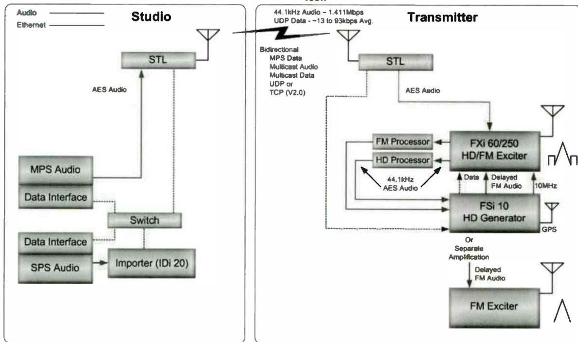
Figure 2: Multicast Architecture, HD Generation at TX Site
