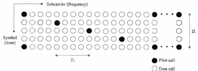
**Figure 2. Pilot pattern in the time-frequency grid**
