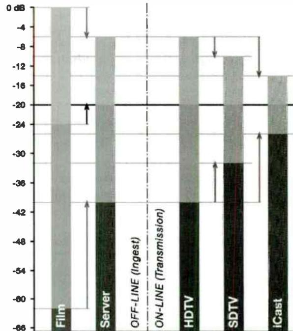
Fig 11. Level transcoding from Film to Broadcast. First align SLM, then process as indicated. Black arrows: Level offset. Red arrows: Dynamics processing.
