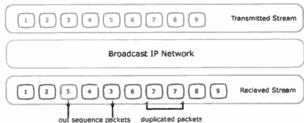
Figure 8 Receive Packet Sequence Errors
