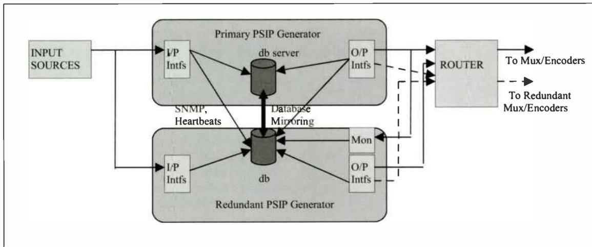
Figure 4. 1+1 redundancy solution
