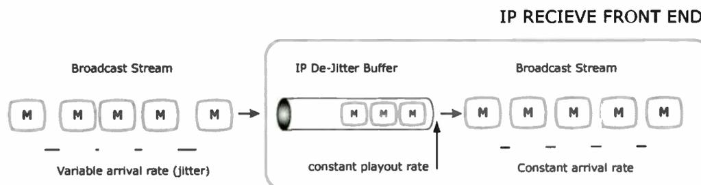
Figure 5 De-Jitter Buffer Model
