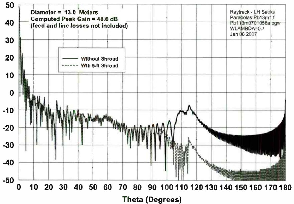
Figure 7 (above). Calculated RPE of 13-m USB uplink dish, zero to  $\pm 180^\circ$  off axis. Courtesy of The Aerospace Corporation (Preliminary).
