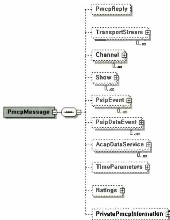
Figure – 7. PMCP Schema for ACAP Data Service
