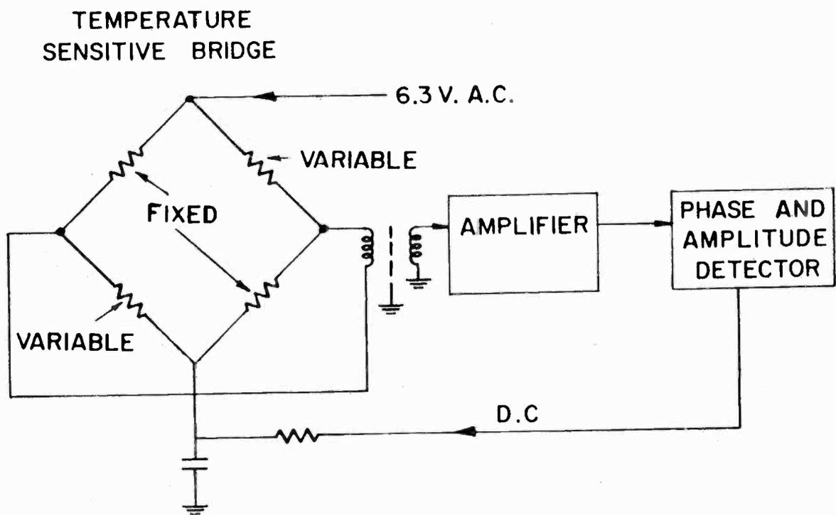
METHOD OF CONTROLLING THE TEMPERATURE OF CRYSTAL OVEN.
