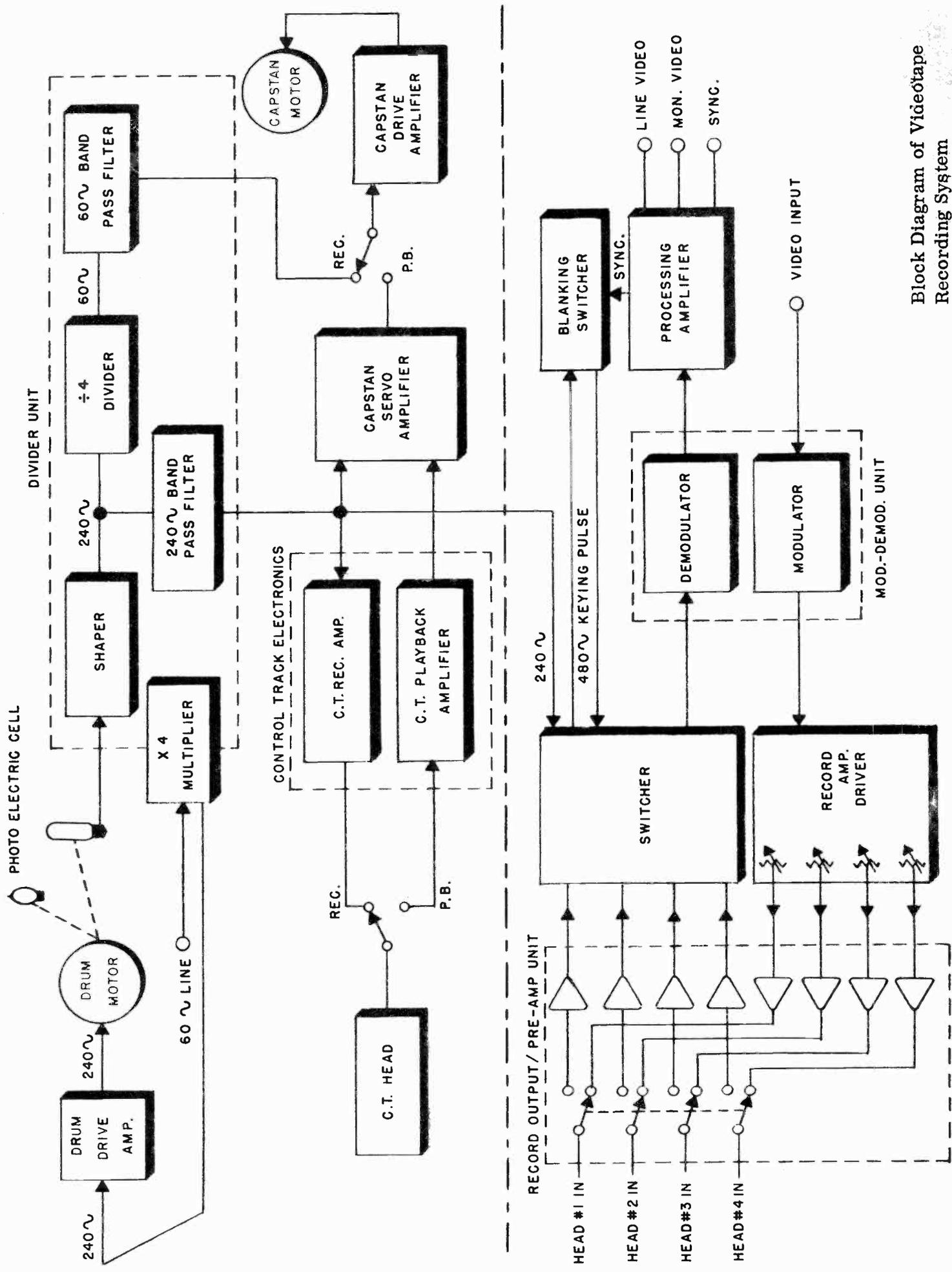
Block Diagram of Videotape Recording System
