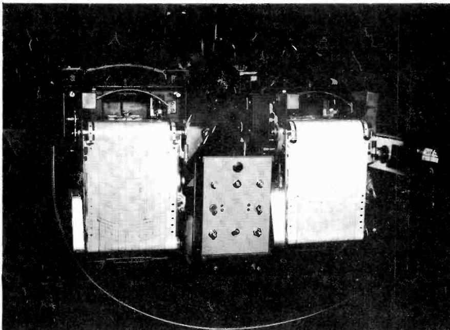
Figure 4 - Chart recorders for mobile unit.
