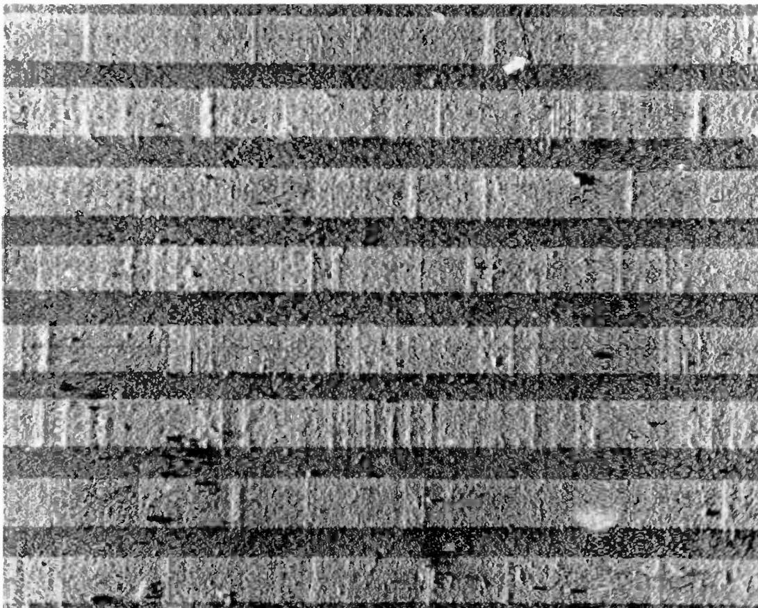
Fig. 9. Photomicrograph of a  $1/8 \times 3/16$  inch area of video tape showing video modulation. (Courtesy of Reeves Soundcraft)
