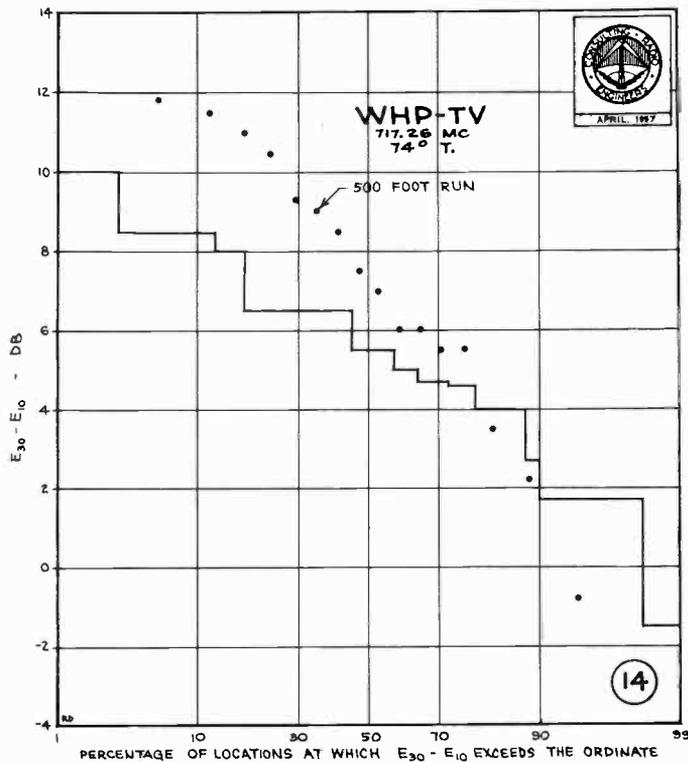
Figure 14 - Distribution of the antenna height-gain function  $E_{30}-E_{10}$  for the measurements of Figure 13.
