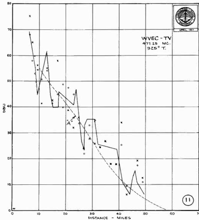
Figure 11 - Continuous 10-foot mobile measurements along the  $325^\circ$  bearing increased by height-gain factors.
