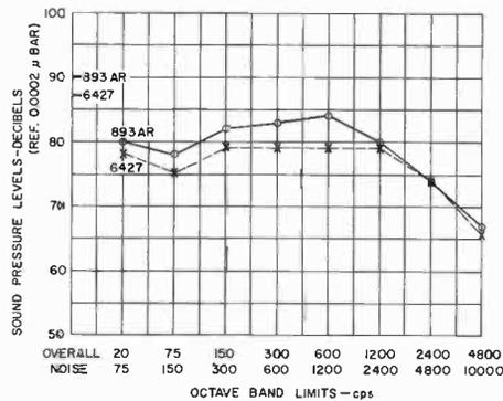
COMPARISON OF AIR NOISE CHARACTERISTICS AT RATES OF AIR FLOW FOR MAXIMUM ANODE DISSIPATION:
