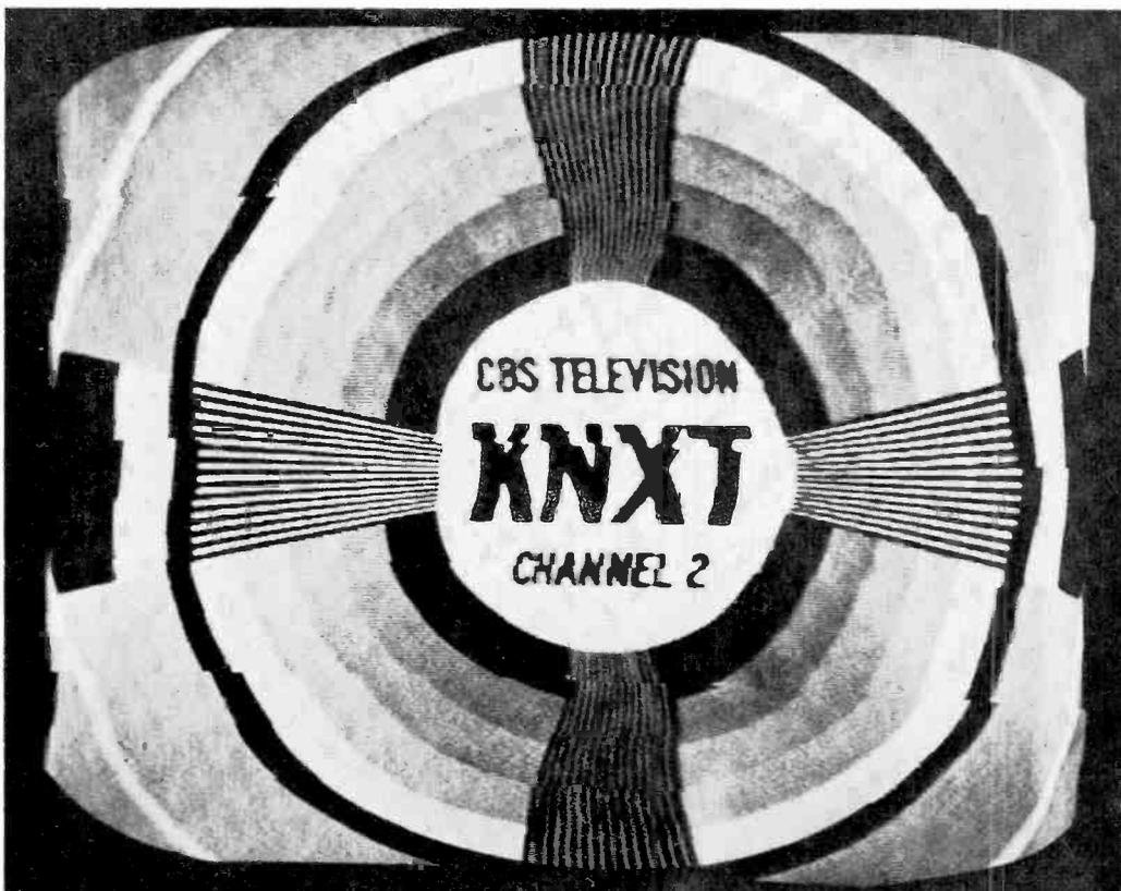
Fig. 6. Picture degradation caused by playing tape back on different head than used for recording.
