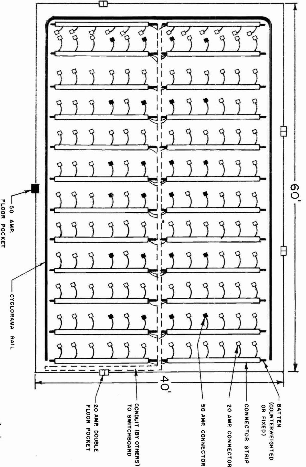
FIG. 1 Typical connector strip layout for a 40' x 60' T.V. Color Studio.
