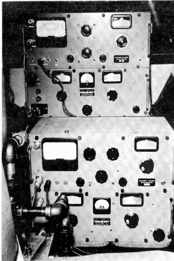
Figure 3 - Interior of mobile unit showing field intensity meters.
