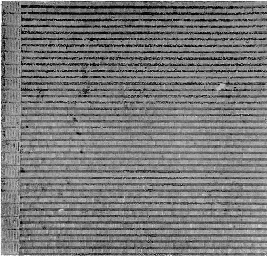
Fig. 8. Photomicrograph of a  $5/8 \times 11/16$  inch area of video tape showing video and control tracks. (Courtesy of Reeves Soundcraft)
