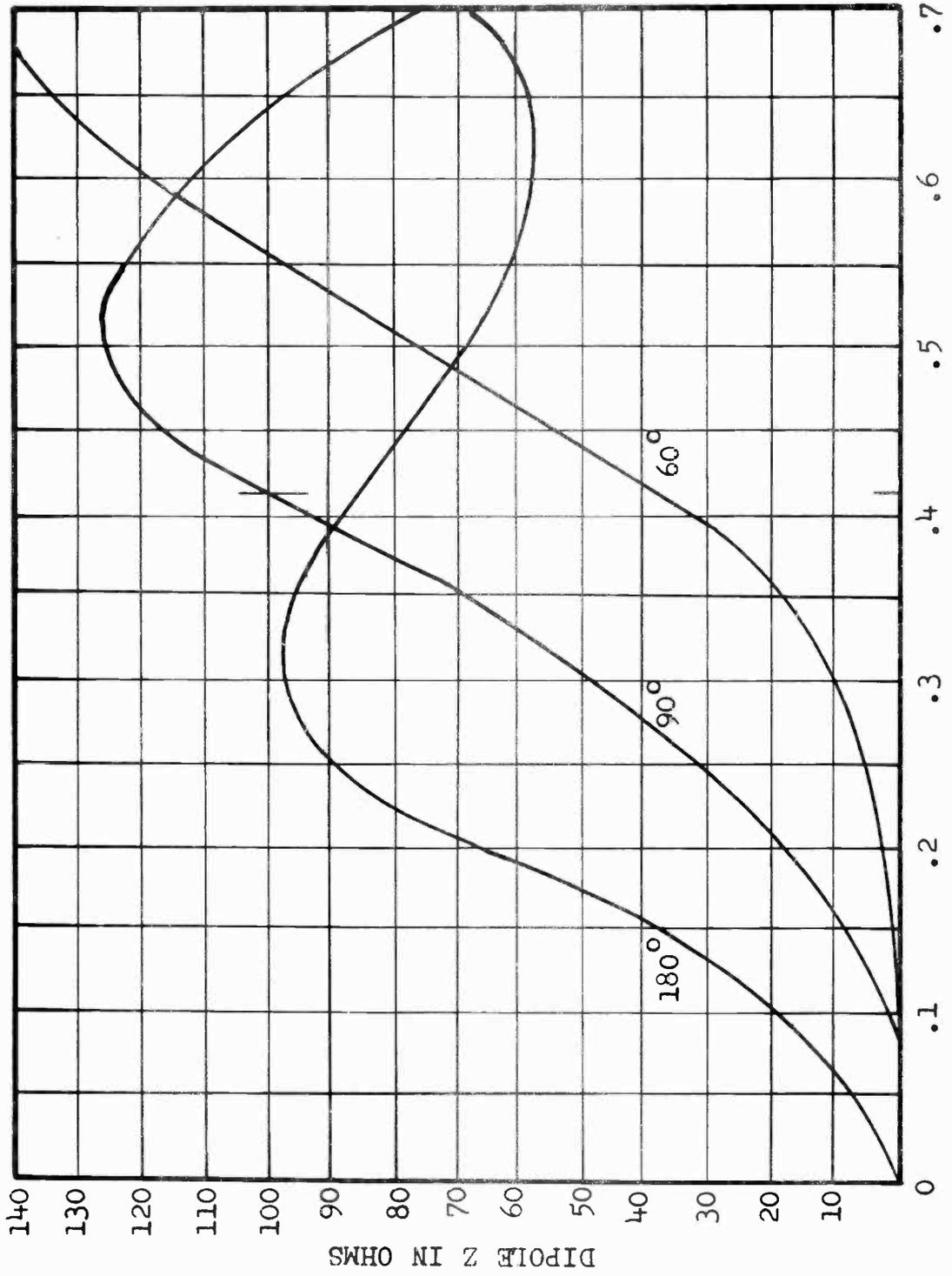
DIPOLE TO CORNER SPACING IN WAVELENGTHS
