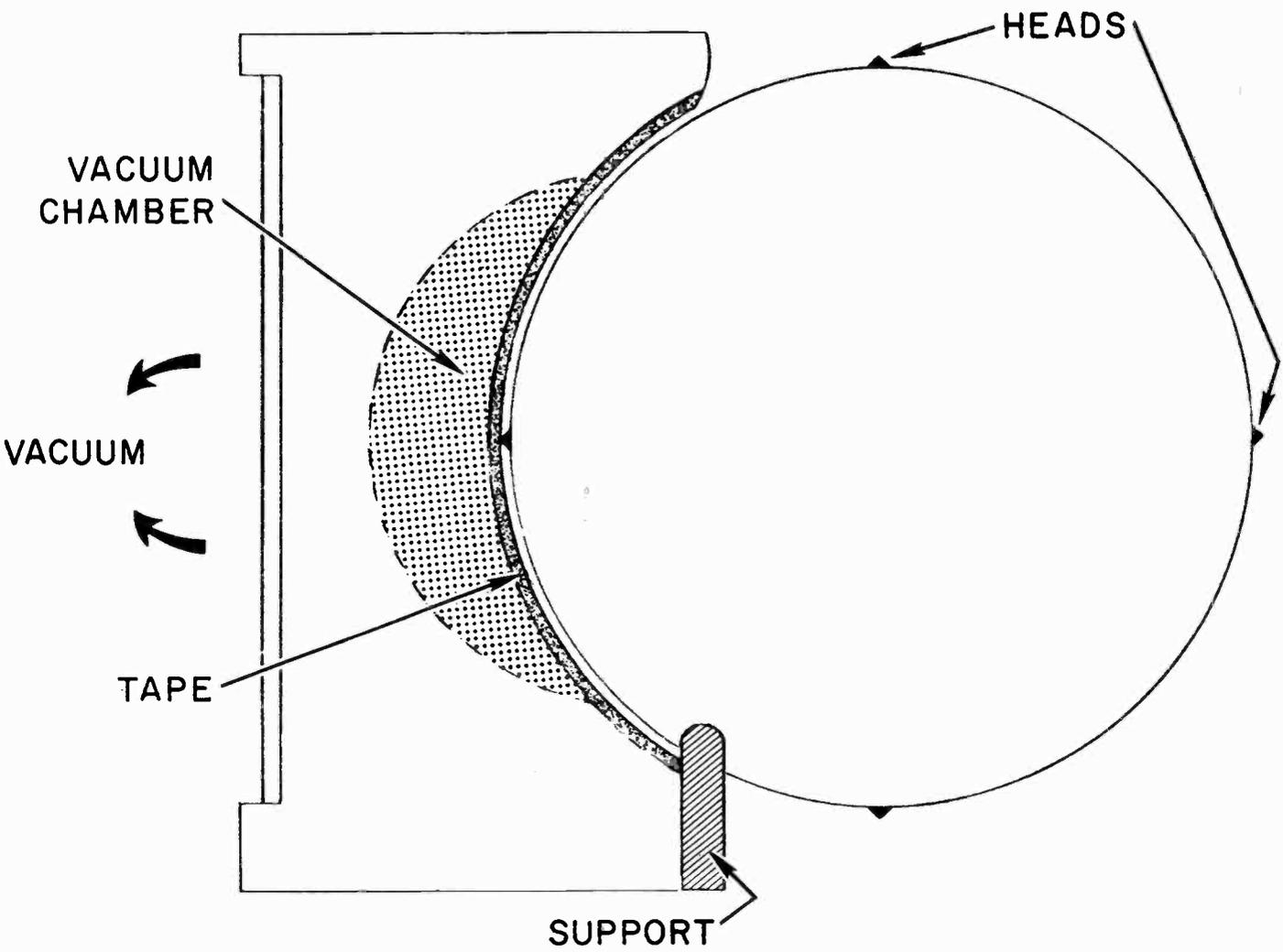
Cross - Sectional Diagram of Rotary
