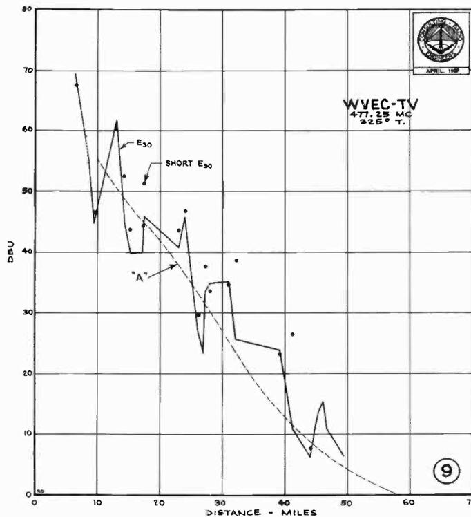
Figure 9 - WVEC-TV field intensities versus distance (reduced to 1 kw radiated) for the  $325^\circ$  bearing.
