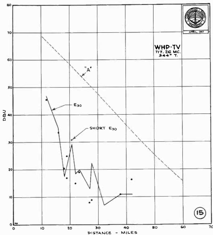
Figure 15 - Plot of 30-foot mobile measurements on WHP-TV on 717.26 mc reduced to 1 kw along a bearing of  $344^{\circ}$  True. The line marked "A" is from FCC Report 2.4.16. This is in very rugged terrain.
