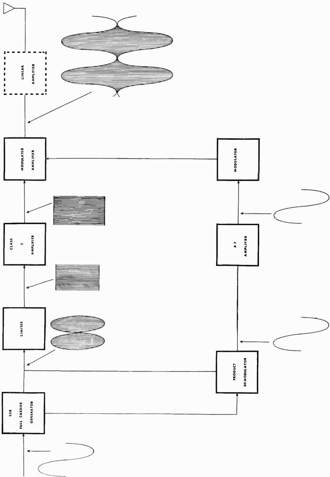
BLOCK DIAGRAM OF BASIC COMPATIBLE SSB SYSTEM
