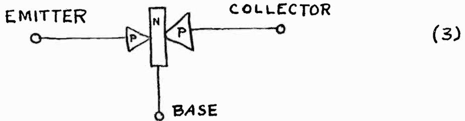
The three elements of the transistor are connected to separate leads, and are labeled emitter, base, and collector, as shown. In a few transistor types of symmetrical design, the emitter and collector have identical properties and may be freely interchanged, but in most transistors the collector junction has a larger area than the emitter junction, leading to differences in electrical characteristics.
