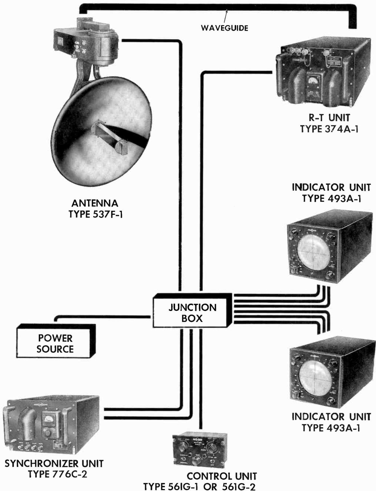
Figure 1. Units of the WP-101 Weather Radar System.
