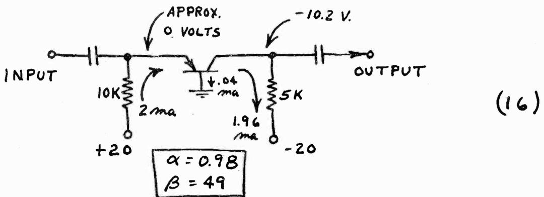
Since the emitter input resistance of only  $40$  ohms is negligible in series with the  $10K$  bias resistor, the emitter bias current is determined by dividing the bias supply voltage ( $20$ ) by the resistance ( $10K$ ), giving  $2\text{ ma}$ . If the transistor
