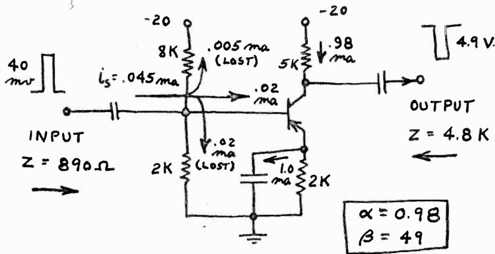
In summary form, the key features of this circuit are: (1) a current gain of about 22, which is less than the beta of the transistor primarily because of the loading effect of the base bias network, (2) a voltage gain of about 122, assuming that the output is not loaded down appreciably by the following stage, (3) a reversal in the polarity of the signal, (4) an input impedance appreciably higher than that of a common-base amplifier, but considerably lower than the 2,000 ohm
