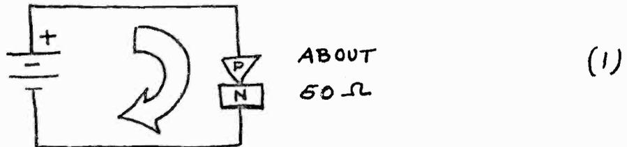
When the battery is connected in the reverse direction, however, the current flow is impeded, and the device appears to have an impedance of the order of 100,000 ohms or more.
