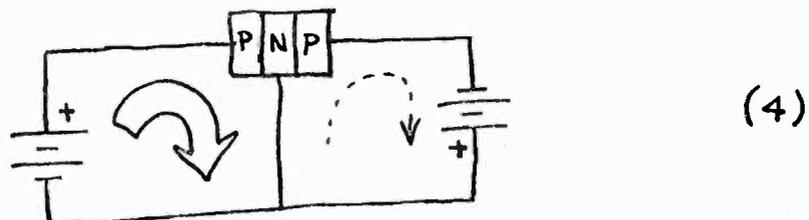
The current through the reverse-biased collector would be very small compared to the emitter current, and the base current would be almost equal to the emitter current. Actually, the situation is almost the reverse:
