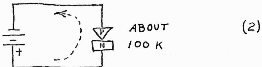
A junction transistor consists, in essence, of two diode junctions in series, with the same very thin piece of N-type material shared by both diode junctions.
