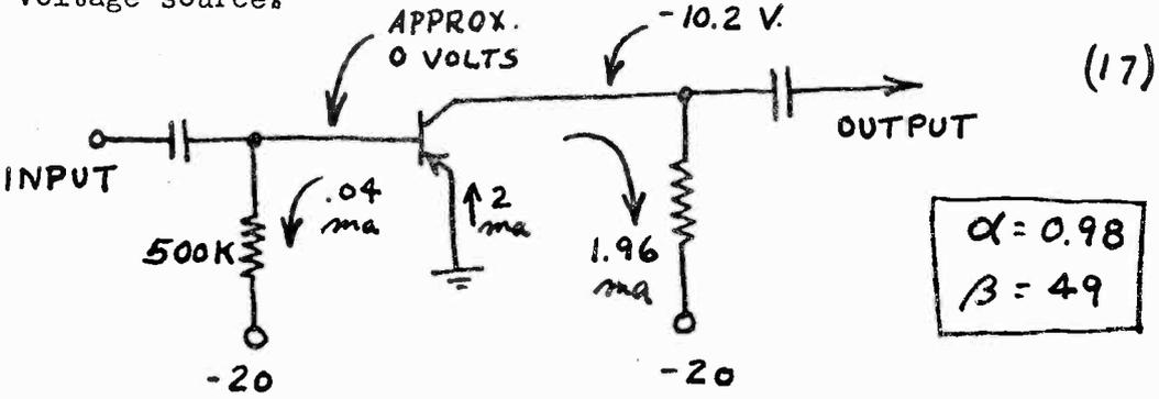
Since the 2,000-ohm input resistance looking into the base of the transistor is negligible in series with the 500K bias resistor, the nominal bias current is determined by dividing the supply voltage (-20V.) by the bias resistance (500K), giving .04 ma in the direction indicated. The collector current is beta times as great, or 1.96 ma, and the collector voltage is determined by subtracting the drop across the load resistor from the supply voltage.
