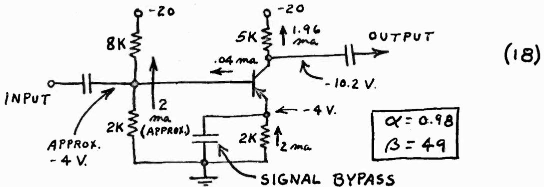
Because of the 2,000-ohm emitter resistance, the d-c resistance looking into the base of the transistor is 102,000 ohms, just as in the case of Figure (15). This high resistance is negligible when shunted across 2,000 ohms, so the current in the voltage divider in the base circuit is nominally equivalent to the supply voltage (-20) divided by the total resistance (10K), or 2 ma. The voltage on
