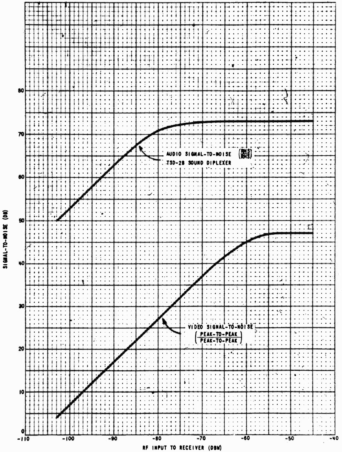
FIGURE 19C - SIGNAL-TO-NOISE RATIO
