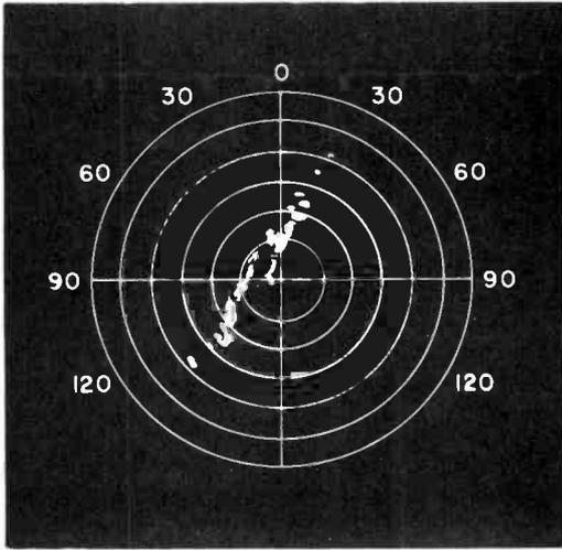
Figure 3. Indicator Display, 150 Mile Range, Initial Detection
