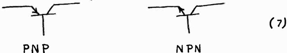
In both cases, the element symbolized by the arrow-head is the emitter, and the direction of the arrow-head indicates the direction of easy current flow.
