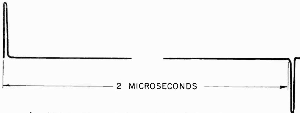
A 1000 FOOT LINE AS SEEN ON A SCOPE WITH D-C PULSE TEST.
