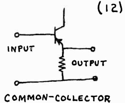
These three basic configurations are superficially equivalent to the vacuum-tube configurations commonly known as grounded-grid, ground-cathode, and cathode follower, respectively.
