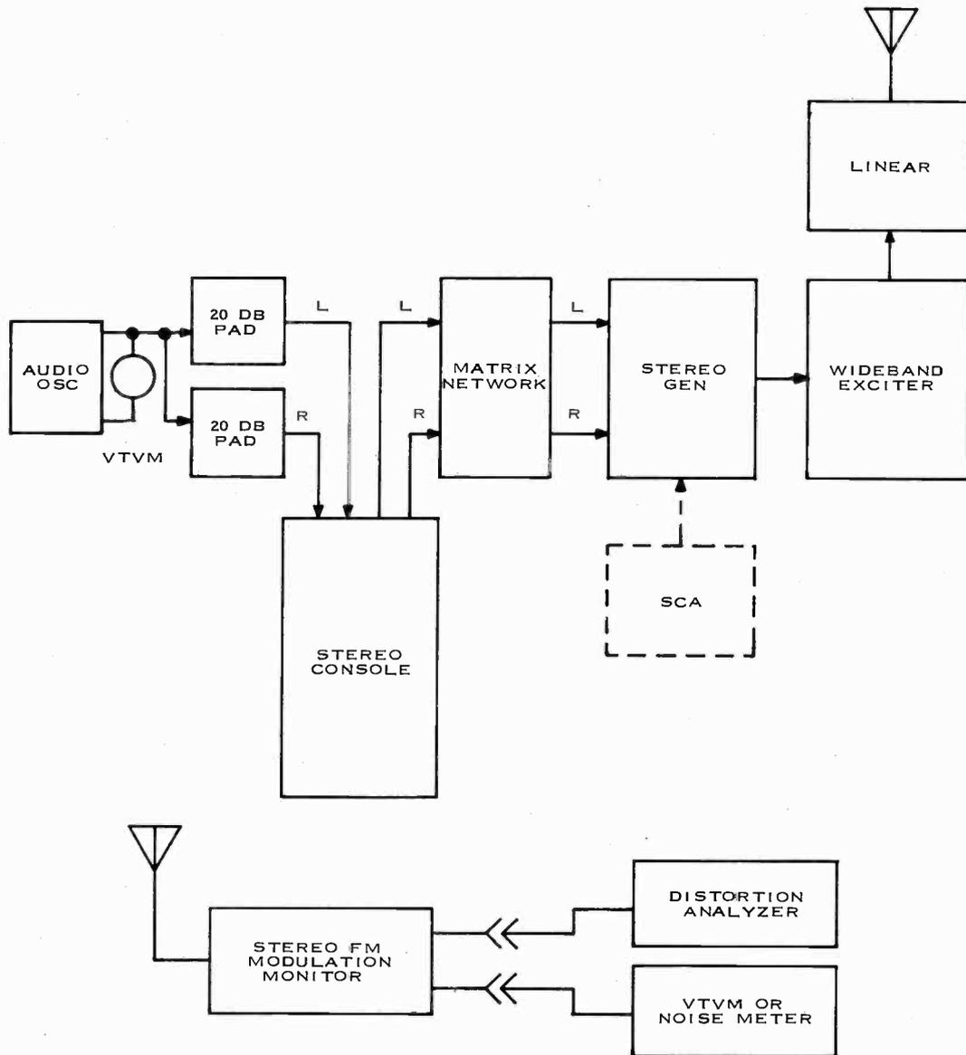
Figure 4. Typical Stereo System and Test Setup
