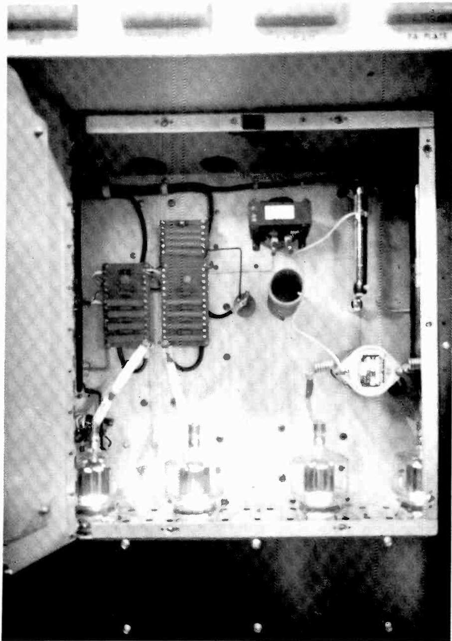
FIG. #5 - TUBES IN 1KW TRANSMITTER NORMAL
