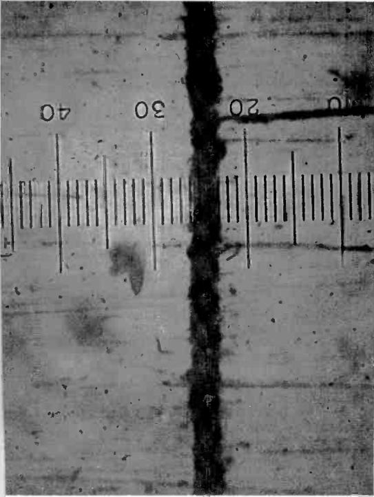
a Gap Photomicrograph (crooked edges)
