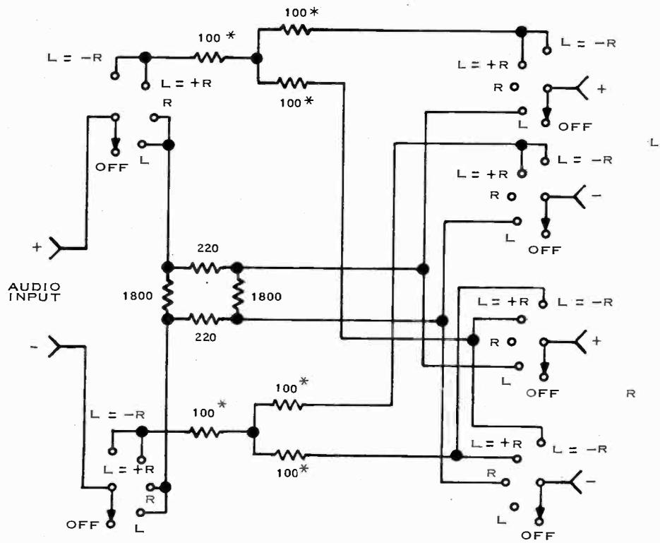
Figure 3. Stereo Test Matrix
