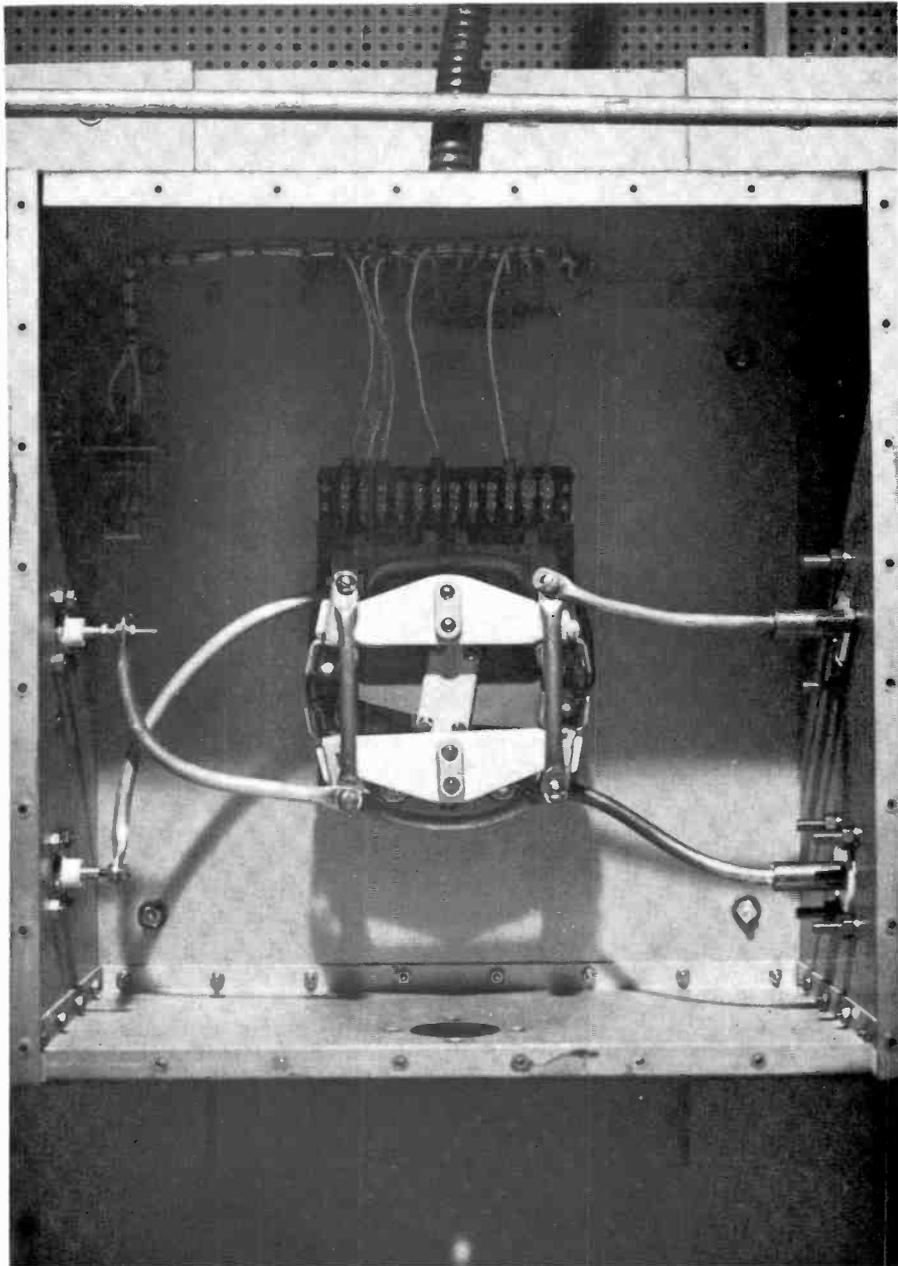
FIG. #9 - ANTENNA RELAY (TRANSFER)
