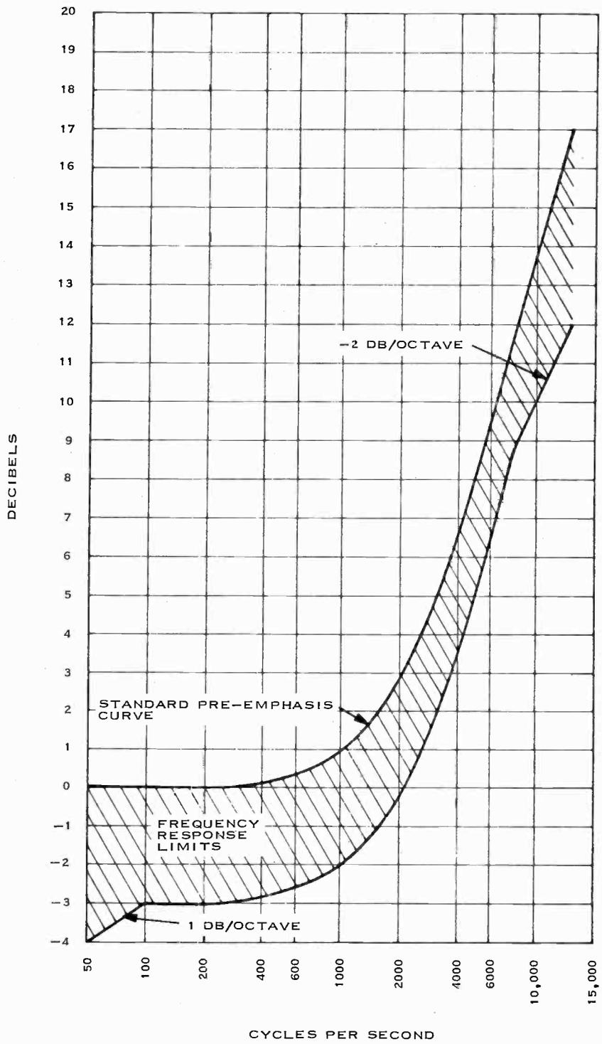
Figure 5. Standard Pre-Emphasis Curve and Frequency Response Limits
