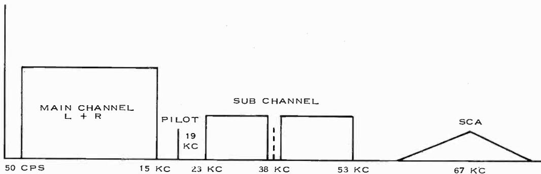
Figure 1. Stereo Multiplex and SCA Frequency Spectrum
