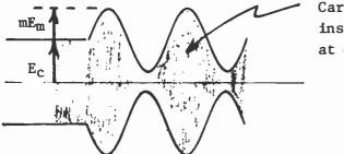
Carrier frequency and phase inside envelope is constant at  $\omega_{\rm C}$  and independent of  $E_{\rm m}$ .
