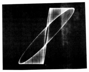
FIGURE 14. LISSAJOUS I.P. M. MEASUREMENT SHOWING 8.6° I.P.M. IN TROUGH AND 17.8° I.P.M. AT CREST OF MODULATION ENVELOPE (90% MODULATION DEPTH)
