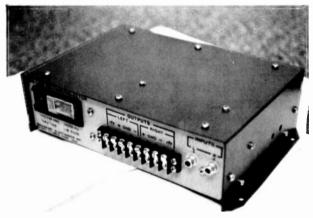
Broadcast Electronics EP-1 Phono Preamp shows extensive RF shielding to minimize both conducted and radiated interference.
