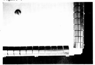
Figure 6 shows fingerstock used on the FM-30 transmitter to provide a positive RF connection betweek the door and the chassis.
