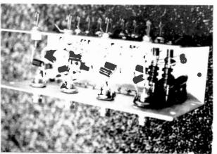
Figure 1 and 2 show the RFI filter assembly from the Broadcast Electronics FX-30 Exciter. All audio and control leads enter the exciter through this assembly. Each lead is filtered by a multi-section filter, with a feedthrough capacitor as a shunt element. This assembly strips off RF energy from the leads before the RF reaches the main cavity of the exciter chassis.
