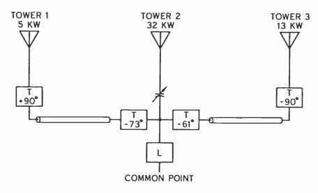
FIGURE 5. PHASOR WITH MINIMUM LOSSES
