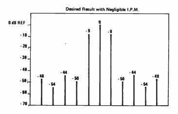
FIGURE 4. RF SPECTRUM OF HYPOTHETICAL TRANS-MITTER HAVING PRACTI-CALLY NO INCIDENTAL PHASE MODULATION AND 2.5% TOTAL HARMONIC DISTORTION.
