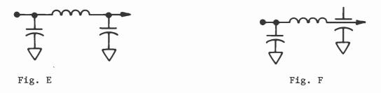
A three element "PI" filter, when components are properly selected, can provide 40 dB of RF attenuation over a wide bandwidth (Fig. E). As with the other two filters above, for good effectiveness at VHF and UHF frequencies, the third element should be a feedthrough capacitor (Fig. F).
