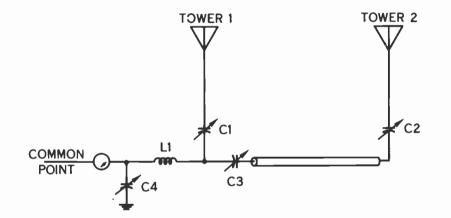
FIGURE 8. PHASOR WITH MINIMUM NUMBER OF COMPONENTS
