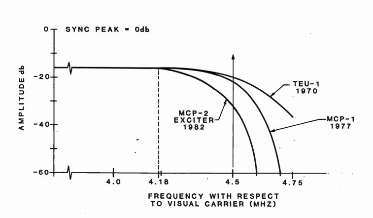
TYPICAL TRANSMISSION AMPLITUDE CHARACTERISTIC NEAR AURAL CARRIER
