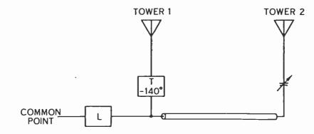
FIGURE 6. PHASOR WITH UNMATCHED TRANSMISSION LINE
