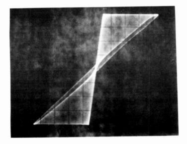
FIGURE 12. LISSAJOUS I.P. M. MEASUREMENT OF AM SIGNAL INDICATING AP-PROXIMATELY 3.8° PEAK PHASE DEVIATION AT MODU-LATION CREST. (80% MODU-LATION) AMPLITUDE OF TROUGH TOO SMALL TO MEA-SURE I.P.M.
