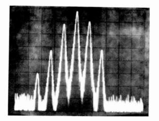
FIGURE 8. RF SPECTRUM OF AM SIGNAL INDICATING VERY EXCESSIVE I.P.M. OF AP-PROXIMATELY 1 RADIAN. NOTE: APPROX. 3dB REDUCTION IN APPARANT CARRIER AMPLI-TUDE (CARRIER SIGNAL IS HIGH SIGNAL ON THE LEFT ) AND VERY HIGH ORDER AND UNBALANCED SIDEBAND PRO-DUCTS. YET AM DISTORTION MEASURES ONLY 1.5%. where:
