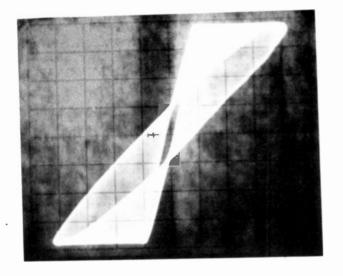
FIGURE 13. LISSAJOUS I.P. M. MEASUREMENT SHOWING 8.6° I.P.M. IN TROUGH AND 13.1° I.P.M. AT CREST OF MODULATION ENVELOPE (75% MODULATION DEPTH)
