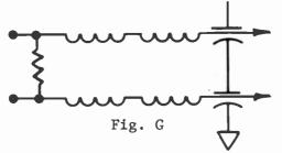
Figure G is an example of a wideband filter used on a balanced audio line. Two inductors are used in series to insure high series impedance over a wide bandwidth. Low impedance feedthrough capacitors insure effective operation into the UHF bands. The 620 ohm resistor was placed in front of the inductors to insure that they do not saturate under high frequency, high level audio signals.
