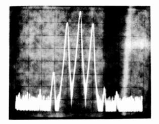
FIGURE 5. RF SPECTRUM OF ACTUAL AM SIGNAL INDICATING PRESENCE OF SMALL AMOUNT OF INCI-DENTAL PHASE MODULA-TION. MEASURED AM DISTORTION OF 1%.
