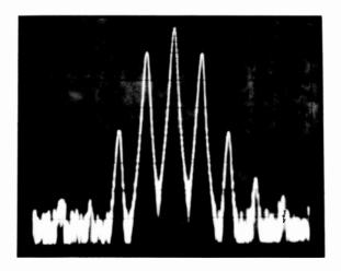
FIGURE 6. RF SPECTRUM OF AM SIGNAL INDI-CATING SIGNIFICANT I.P.M. NOTE: 2nd ORDER SIDEBANDS ONLY 30db BELOW 1st ORDER SIDE-BANDS YET AM DISTOR-TIONS MEASURES 1%.
