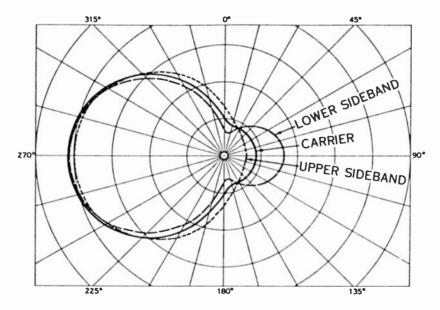
FIGURE 4. EXAMPLE OF POOR PATTERN BANDWIDTH
