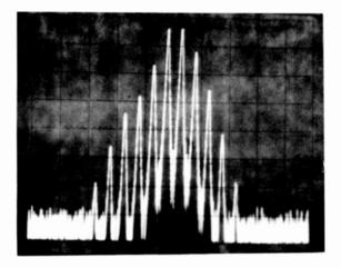
FIGURE 7. RF SPECTRUM OF AM SIGNAL INDICATING PRESENCE OF APPROX. 20<sup>O</sup> OF PEAK PHASE MODULATION. NOTE: THE 1dB REDUCTION IN APPARANT CARRIER AMPLI-TUDE AND 2nd ORDER SIDE-BANDS ONLY 20dB BELOW DE-SIRED SIDEBANDS YET AM DISTORTION MEASURES 1%.
