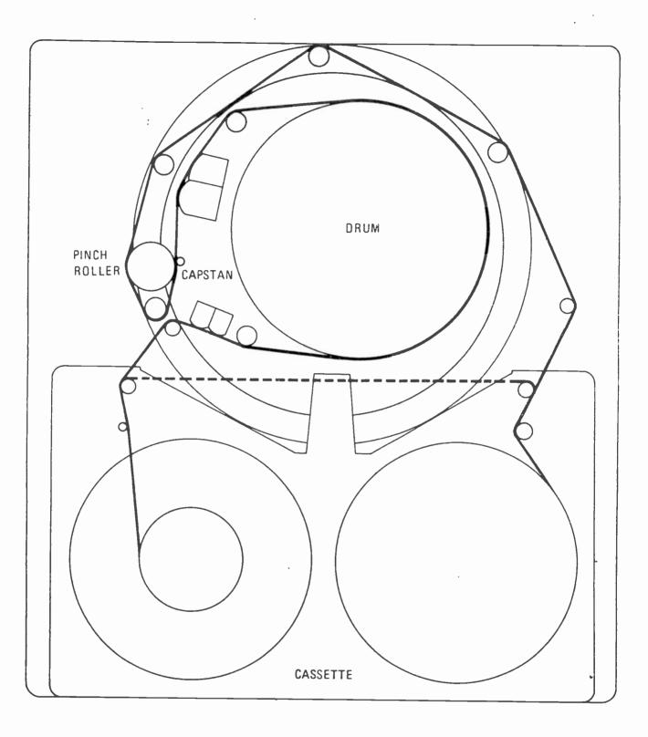
Fig. 1. RELATIONSHIP OF CASSETTE, DRUM, LOADING MECHANISM AND THE SIZE OF VTR MECHANISM
