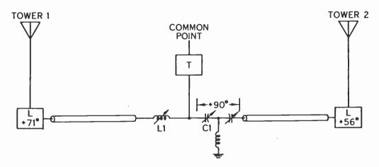
FIGURE 7. PHASOR WITH LEADING L NETWORKS AT TOWERS AND BACK-TO-BACK PHASE AND RATIO CONTROL
