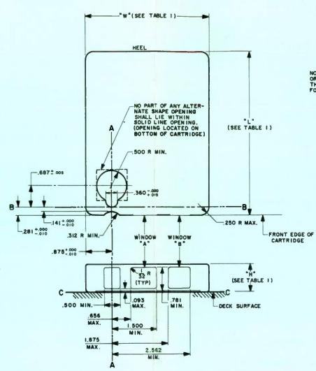
FIG. 3 CARTRIDGE DIMENSIONS
