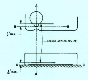
FIG. I REQUIRED SPRING ACTION DEVICE LIMITATIONS
