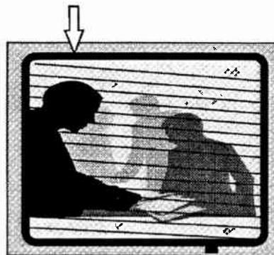
Video Signals are transmitted at 30 frames per second with 2 vertical scans per frame = 60 vertical scans per second.
