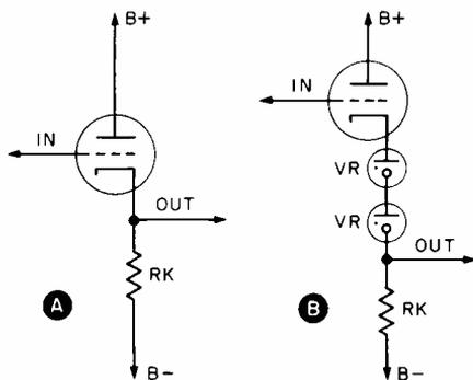
FIG. 4. Typical single ended output circuits.
