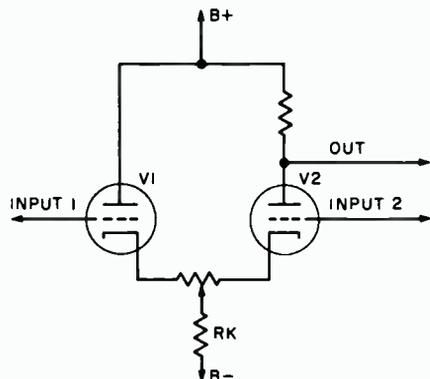
FIG. 3. Basic differential amplifier.
