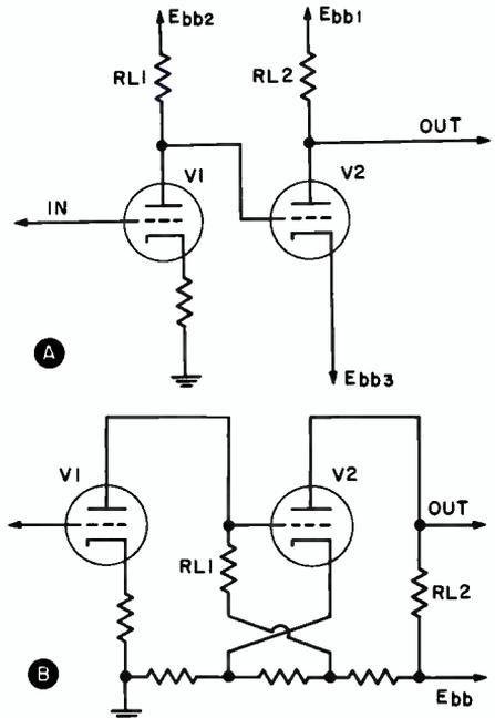
FIG. 1. Simple two stage dc amplifiers.
