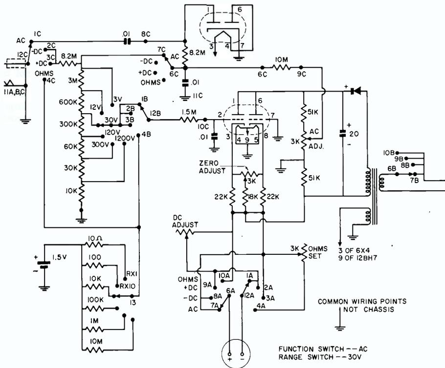
FIG. 6. Complete Diagram of CONAR 211.
