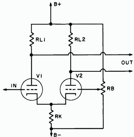
FIG. 2. Basic cathode coupled input stage.
