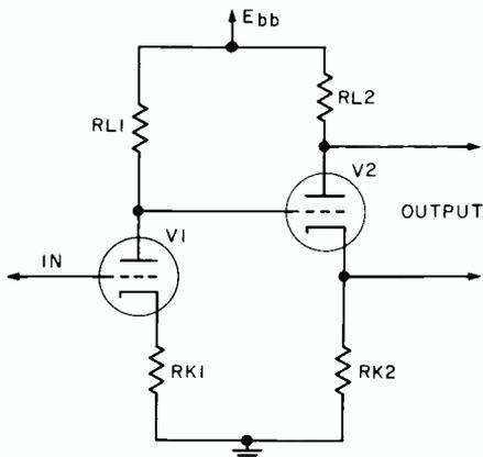
FIG. 7. Direct coupled phase inverter.
