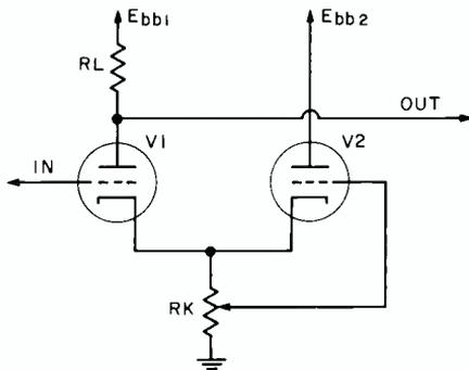
FIG. 8. Using a second tube for heater compensation.
