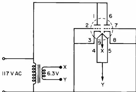
FIG. 5. Circuit for curing bridge tube.
