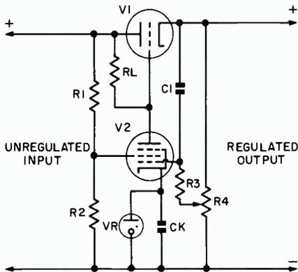
FIG. 5. Degenerative series voltage regulator.
