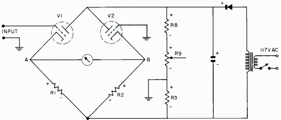
FIG. 1. Power Supply -- bridge circuit.
