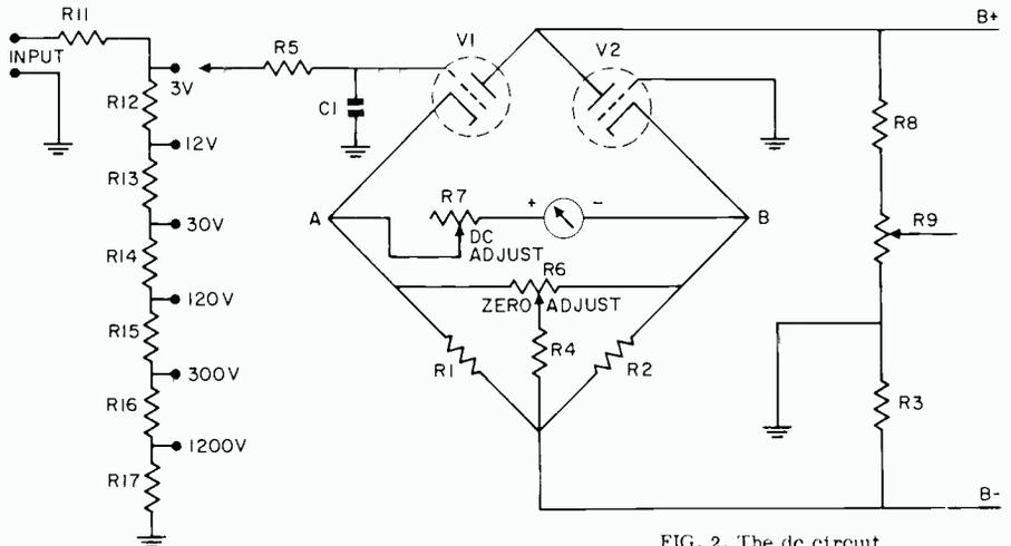
FIG. 2. The dc circuit.
