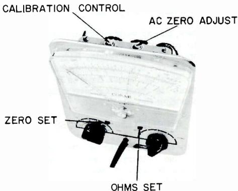
Model 211 VTVM showing the calibration controls.
