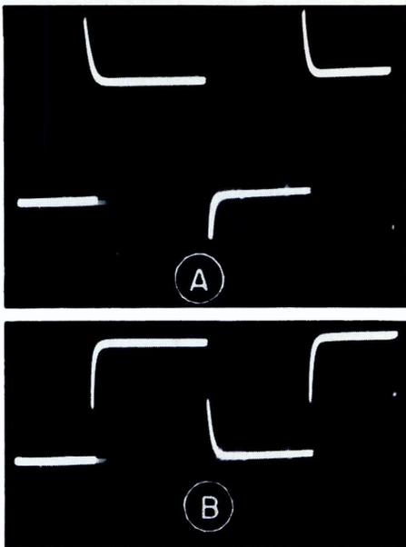
FIG. 5. Square wave distortion caused by improperly set frequency compensating capacitors.
