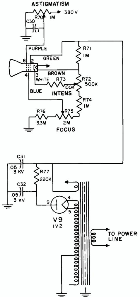
FIG. 2. 1V2 power supply and connections to crt.
