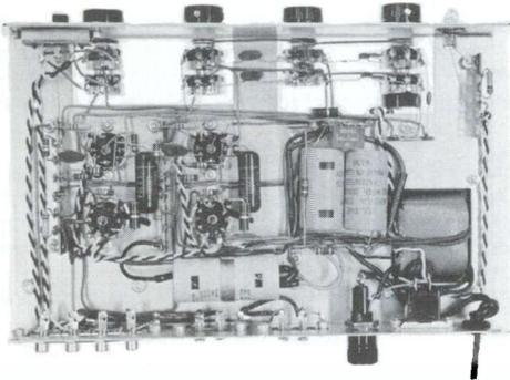
FIG. 2. Photo showing chassis wiring of the amplifier.
