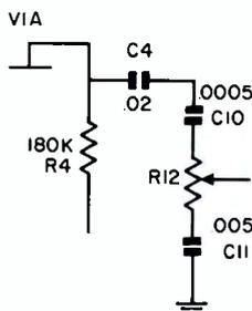
FIG. 5. Treble circuit.
