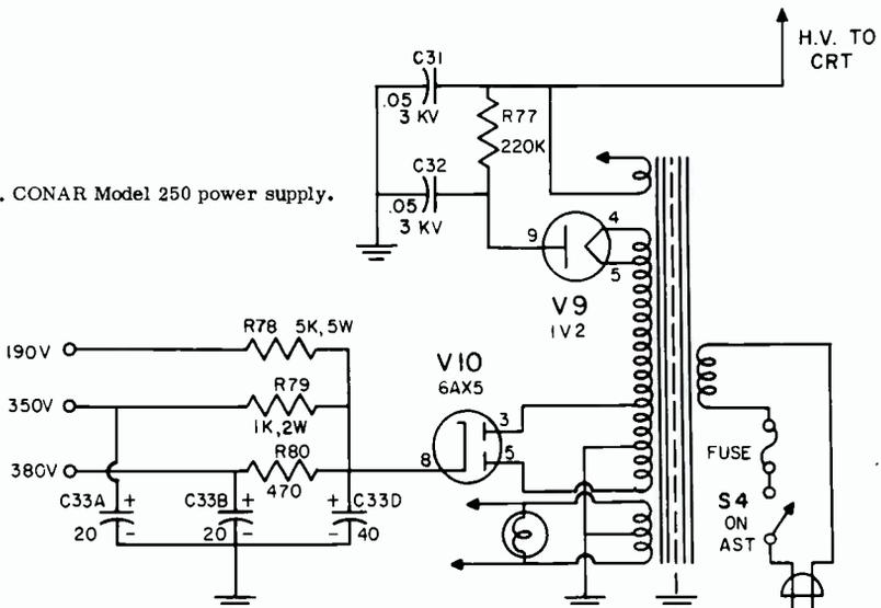
ages obtained from the low-voltage supply. Lower than normal voltage at one of these outputs indicates a defect in the scope that is loading that circuit. The defect may be a shorted tube or capacitor. You can check tubes simply by removing them, capacitors by disconnecting one of their leads. If you cannot find a defect which is placing an excessive load on the power supply, the chances are the input filter capacitor is defective.
