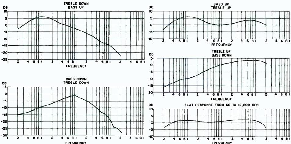
FIG. 3. Response curve shapes available by adjusting the bass and treble controls.
