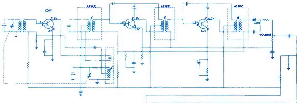
FIG. 3. Schematic diagram of a typical transistor portable receiver.
