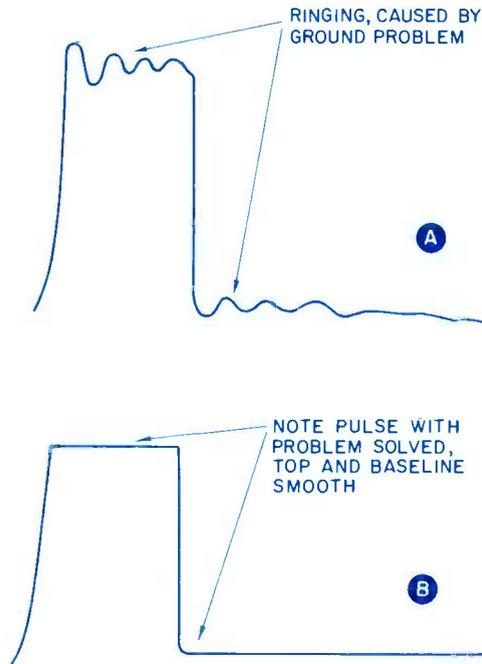
FIG. 2. (A) Pulse with damped oscillations on top and baseline. (B) Corrected pulse.
