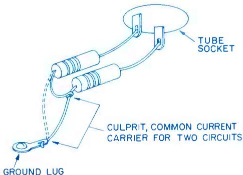
FIG. 4. Resistors connected between tube circuits and ground lug showing source of ground problem. The dotted line indicates a possible method of correcting the problem.
