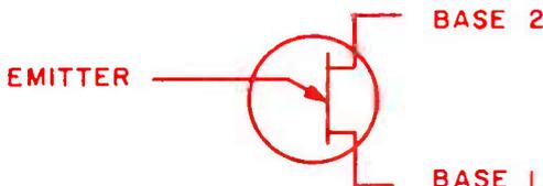
Note the emitter and two bases as we mentioned earlier. The controlling element is schematically represented on
