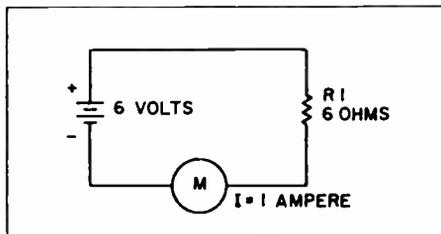
FIG. 1. A simple dc circuit.
