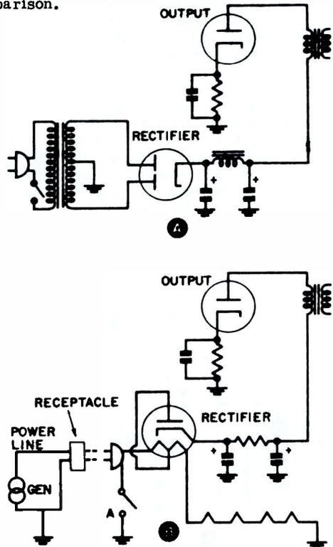
FIG. 3. Power supplies. A, ac; B, ac-dc.
