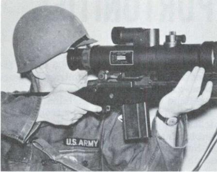
Light-amplifying tubes that permit soldiers to see in the dark without their own presences being revealed will be produced in Springdale, Conn., for the U. S. Army by the Machlett Laboratories, Inc. (subsidiary of the Raytheon Co.). The tubes intensify the natural low level of night illumination to present a bright image, thus providing the soldier with fire power and mobility comparable to daytime levels.
