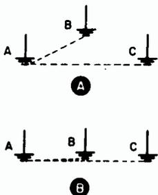
FIG. 9. A, right ground connection; B, wrong.
