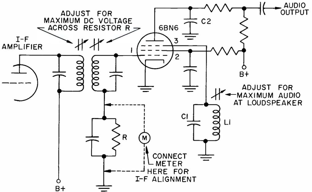
FIG. 2. Gated-beam FM detector/limiter/audio amplifier.
