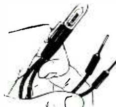
Test voltage in any circuit. Indicator shows when circuit is hot. AC or DC 90 to 500 volts. Clip on shirt or coat pocket.
