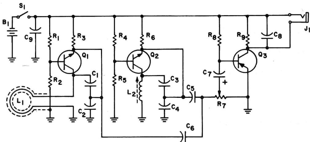
Fig. 1. Schematic of the metal detector.
