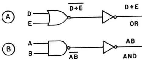
Fig. 5. Generating AND and OR functions with NAND/NOR gates.
