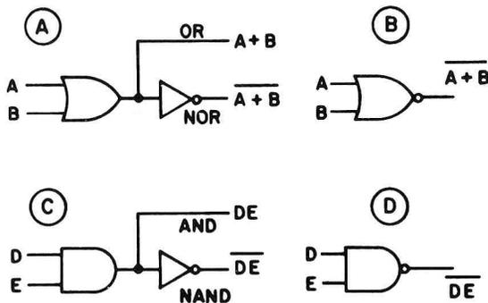
Fig. 1. How NAND/NOR gates are formed and designated with symbols.
