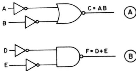
Fig. 6. Performing the AND operation with a NOR gate is shown at (A); performing the OR operation with a NAND gate is shown at (B).
