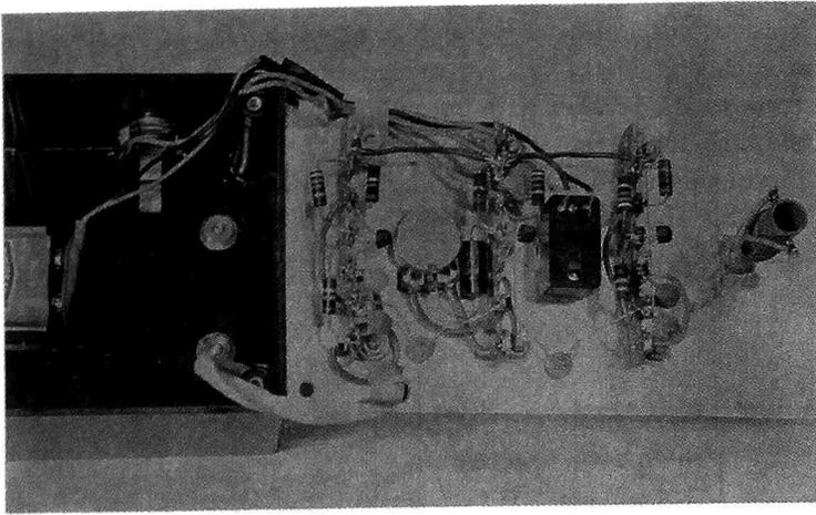
Fig. 3. Connections between top cover and box.
