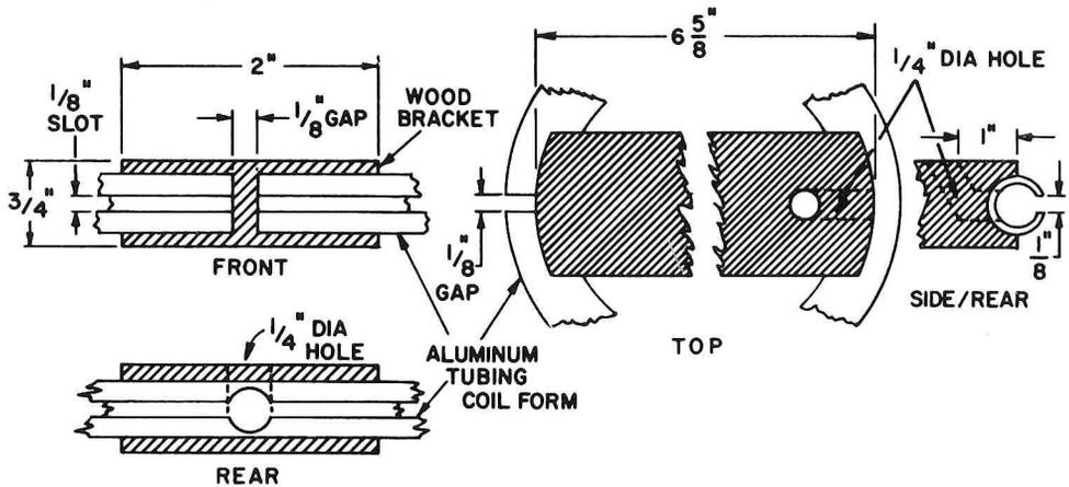
Fig. 4. Construction of search coil.
