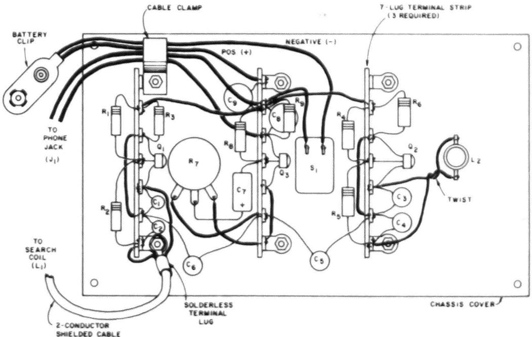
Fig. 2. Circuit layout.
