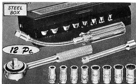
**12-PC. 1/4" DRIVE SOCKET SET:** Complete set includes: 8-pc. hex drive socket set—3/16" to 7/16"; 5 1/2" reversible ratchet with 1/4" drive, 3 1/2" extension bar; flexible shaft handle; sturdy steel carrying box.
