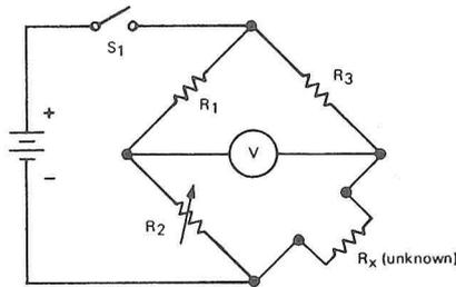
Here an unknown resistance,  $R_x$ , is connected as one of the arms of the bridge. Arm  $R_2$  is made variable. When power is applied by closing switch  $S_1$ , the circuit operates.  $R_2$  is adjusted until balance is obtained. At this time, we know that:
