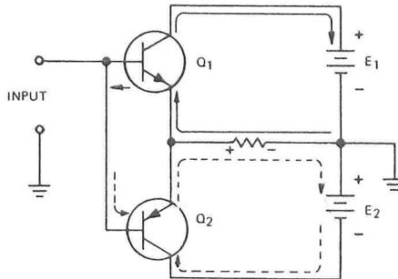
This circuit is basically an emitter follower or common collector amplifier since the load is in the emitter circuit. But complementary symmetry amplifiers with a common emitter connection can also be constructed.
