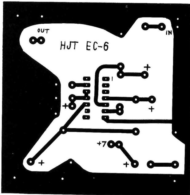
Fig. 6. Actual size foil pattern for 723 audio amplifier.
