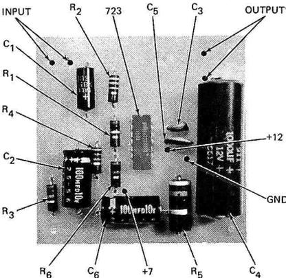
Fig. 8. Location of all parts mounted to the circuit board.
