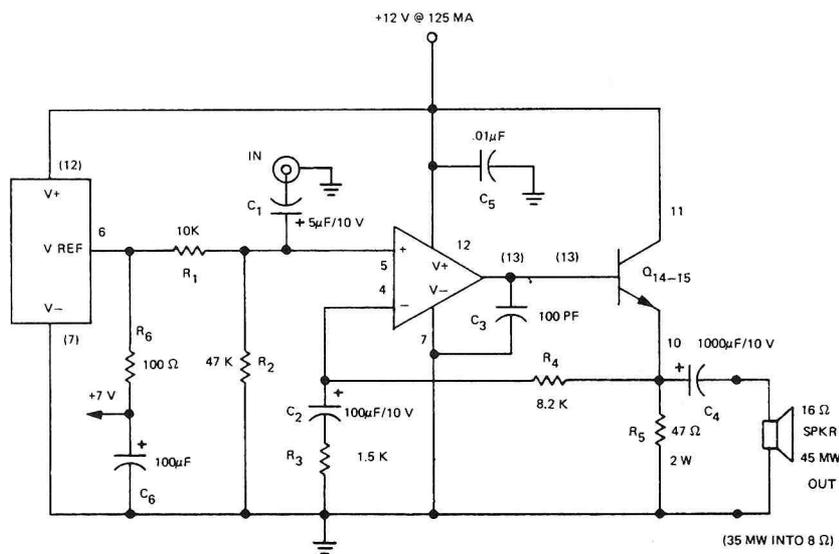
Fig. 5. Typical power supply circuit converted to an audio power amplifier.
