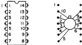
Fig. 7. DIP circuit board pattern that suits either DIP or "TO-5" package.
