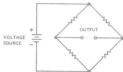
It consists of an input voltage source, four elements or arms, and an output. For simplicity, we have shown a battery as a voltage source; however, any dc or ac voltage source can be used. The elements, or arms, shown here are resistors; but as you will see, practically any other electronic component can be used as well. A load resistor or indicating device such as a meter is usually connected to the output.
