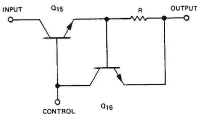
Fig. 3. Simple current limiter circuit.
