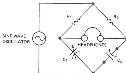
The sine wave signal source applies an audio signal to the bridge. Capacitor  $C_x$  has an unknown value. Calibrated capacitor  $C_1$  is varied until a balance is obtained. Then the value of  $C_x$  can be read from the dial.
