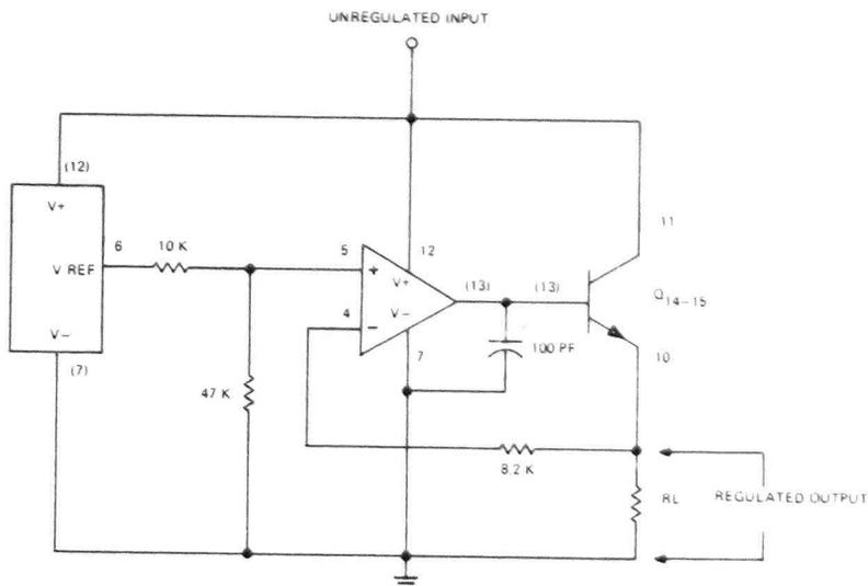
Fig. 4. Basic 723 voltage regulator circuit output — 6 V @ 150 MA maximum.
