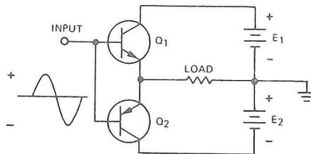
This is a push-pull class B power amplifier known as a complementary symmetry circuit. The term complementary comes from the use of transistors with equivalent characteristics but of opposite sex.  $Q_1$  is an NPN,  $Q_2$  is a PNP.
