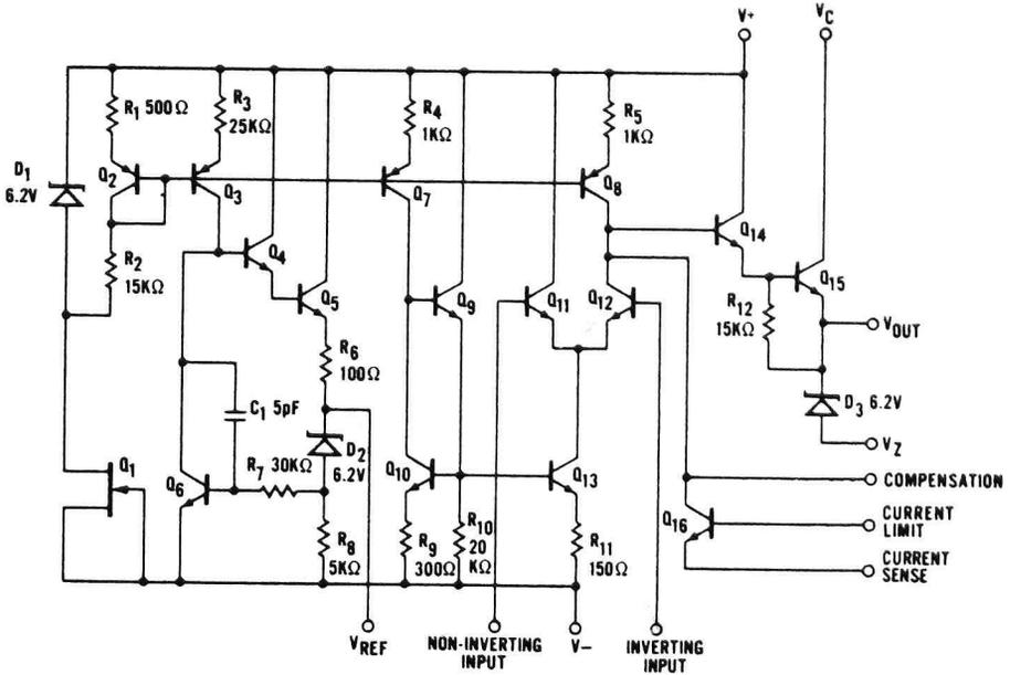
Fig. 1. Internal schematic of a 723 voltage regulator. (Courtesy Fairchild Semiconductor)
