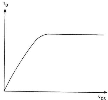
Fig. 2. Characteristic curve of FET.
