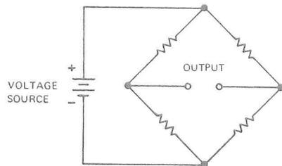
It consists of an input voltage source, four elements or arms, and an output. For simplicity, we have shown a battery as a voltage source; however, any dc or ac voltage source can be used. The elements, or arms, shown here are resistors; but as you will see, practically any other electronic component can be used as well. A load resistor or indicating device such as a meter is usually connected to the output.
