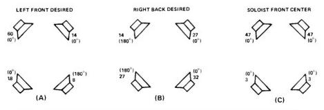
FIGURE 4. POWER AND PHASE DISTRIBUTION FOR THE "OLD" EV DECODER.
