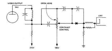
FIGURE 1. SIMPLIFIED SCHEMATIC SHOWING BREAK IN CONTRAST CONTROL.
