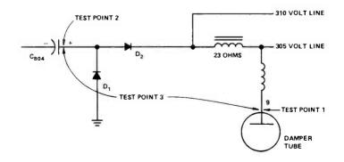
FIGURE 2. SIMPLIFIED SCHEMATIC SHOWING TEST POINTS.
