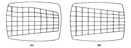
FIGURE 5. KEYSTONING DUE TO A BROKEN CORE (A) AND DUE TO A SHORTED WINDING (B).
