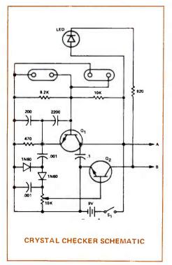
I decided to put in two crystal sockets so that I could plug in either FT-243 or HC-6 type crystals. With the values shown in the schematic, the circuit should oscillate very nicely with crystals from about 1 MHz to 15 or 20 MHz fundamental frequencies. If you go outside of this range you will probably have to play with the values of the emitter resistor and the two capacitors in the base circuit of  $Q_1$ .
