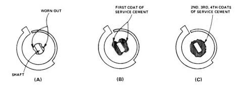
FIGURE 6. WAFER REPAIR.
