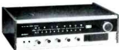
Dual front and rear bass, treble, and balance controls—tape monitor—two head-phone jacks—FET/IC tuner—power bandwidth: 20-20,000 Hz. Dimensions: 4-3/4 by 16-3/8 by 11-1/2. 117 volts ac.
