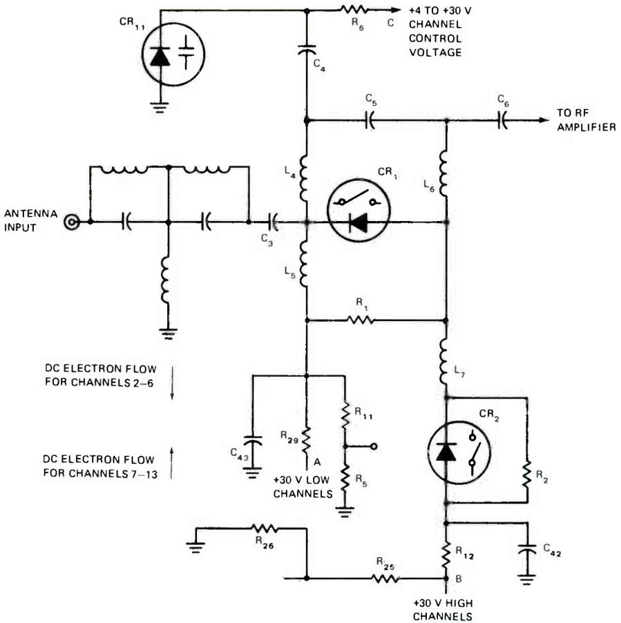
FIGURE 3. (A) INPUT CIRCUIT OF RCA KRK 155 TUNER. (B) EQUIVALENT RESONANT CIRCUIT FOR CHANNELS 2-6.
