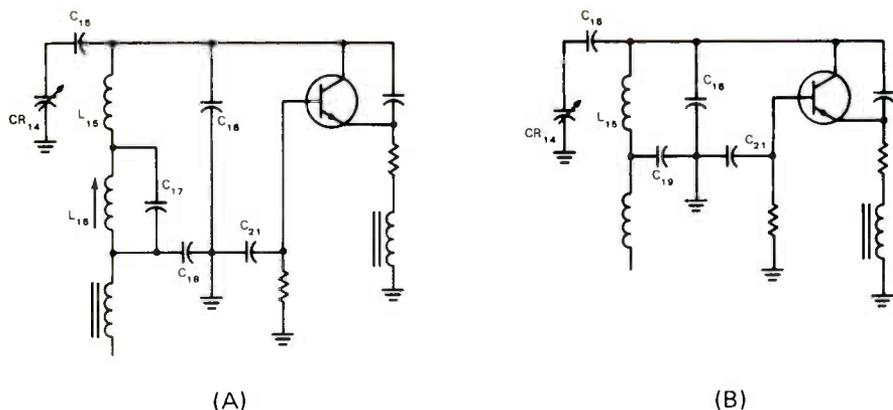
FIGURE 5. THE OSCILLATOR EQUIVALENT TANK CIRCUITS FOR RCA KRK 155 VHF TUNER. (A) CHANNELS 2-6. (B) CHANNELS 7-13.
