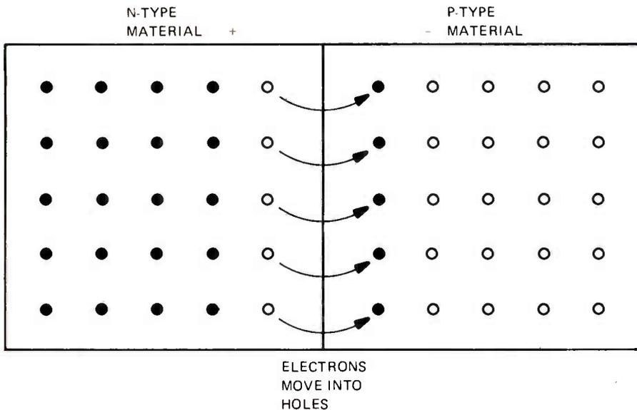
FIGURE 1. DISTRIBUTION OF CARRIERS IN A JUNCTION DIODE.
