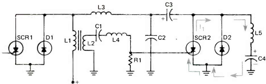
**FIGURE 6. CURRENT FLOW AT THE START OF THE SECOND HALF OF THE TRACE CYCLE, JUST AFTER T2.**
