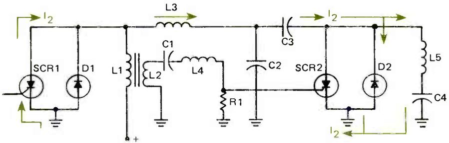
**FIGURE 8. CURRENT FLOW DURING THE INTERVAL T4 TO T5 WHEN SCR1 AND D2 ARE CONDUCTING.**
