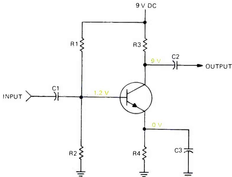
FIGURE 4. A NONCONDUCTING (CUT OFF) TRANSISTOR.
