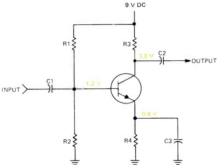
FIGURE 5. A LEAKY TRANSISTOR.
