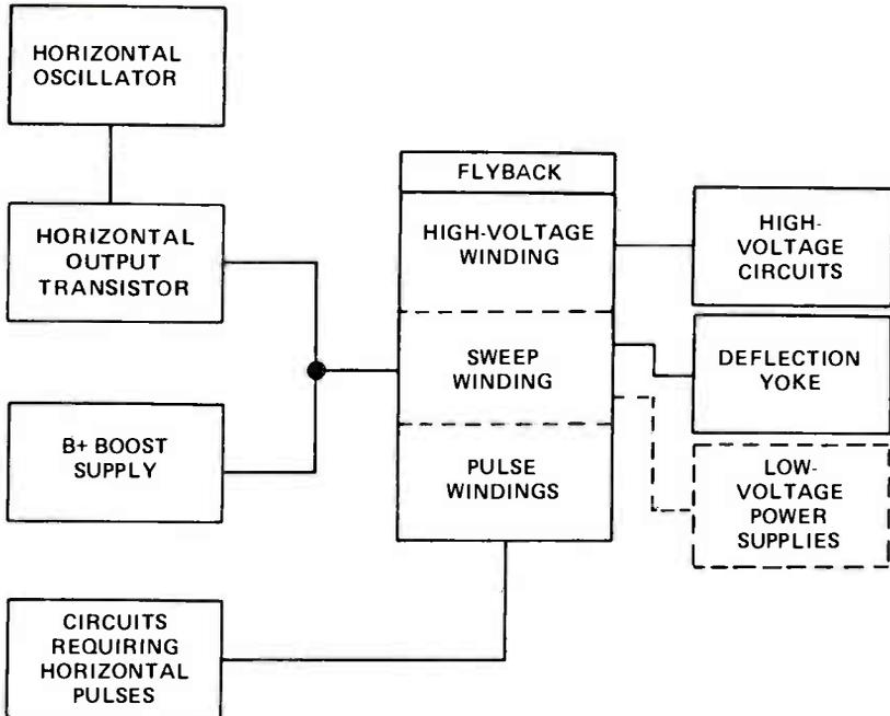
FIGURE 1. THE HORIZONTAL CIRCUIT HAS MANY ADD-ONS, MAKING IT THE MAJOR POWER-CONSUMING CIRCUIT IN THE TELEVISION RECEIVER.
