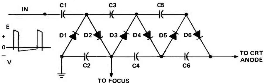
FIGURE 3. AN INTERNAL LOOK AT THE HIGH-VOLTAGE TRIPLER.
