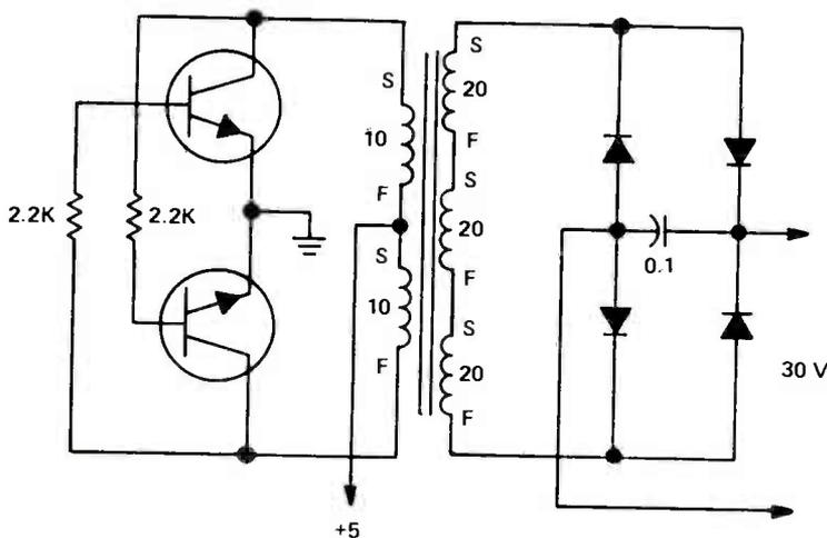
FIGURE 1. DC-TO-DC CONVERTER USING A HOMEMADE TOROID TRANSFORMER.
