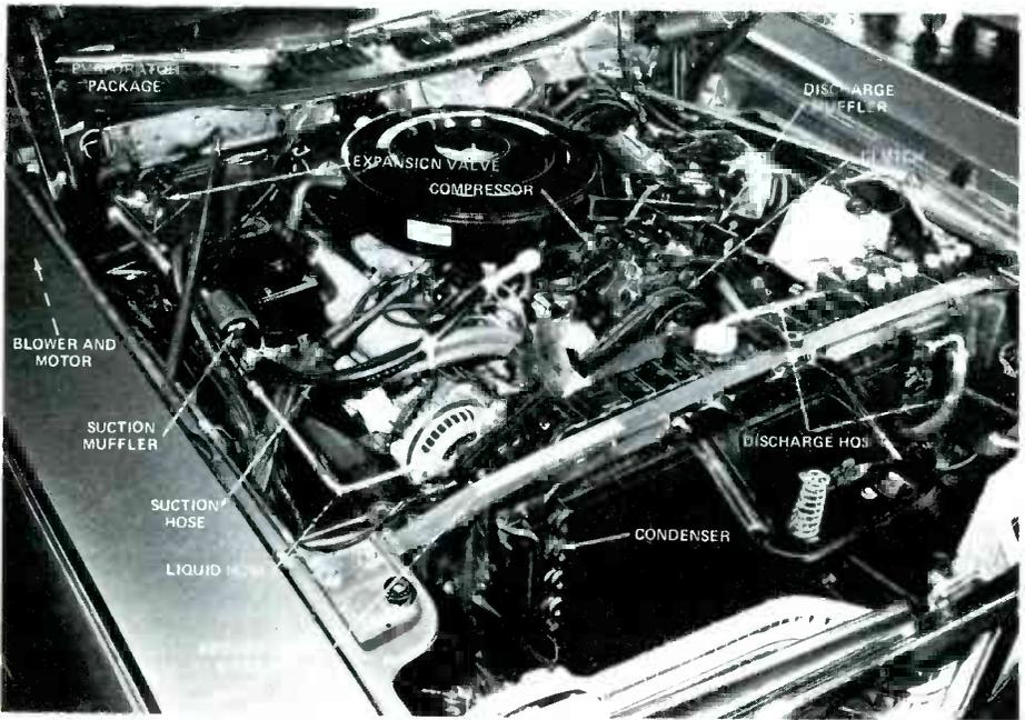
FIGURE 1. AIR-CONDITIONING COMPONENTS LOCATED IN THE ENGINE COMPARTMENT.
