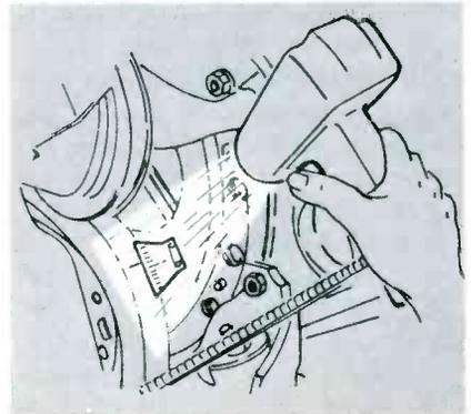
FIGURE 5. TIMING THE IGNITION.
