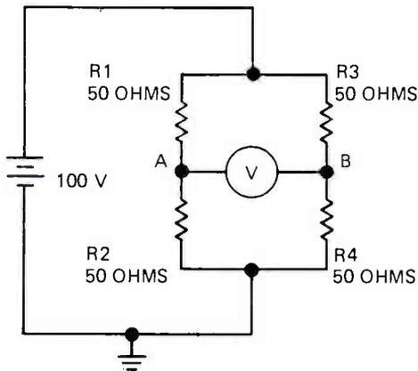
FIGURE 1. A BASIC WHEATSTONE BRIDGE CIRCUIT.
