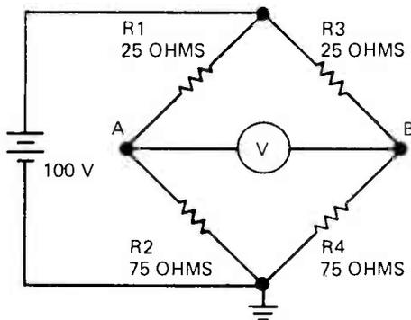
FIGURE 2. THE BASIC BRIDGE CIRCUIT IN ITS MORE CONVENTIONAL FORM.
