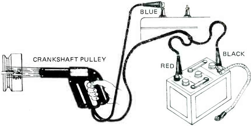
FIGURE 4. A TIMING LIGHT IS USED TO CHECK IGNITION TIMING.
