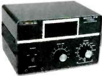
Exclusively from CONAR . . . A superb instrument for the electronics technician, with solid-state circuitry and digital readout. The Model 312 uses two 7-segment LED displays visible through a window in the front panel — a foolproof method for determining the unknown value of a resistor or capacitor.
