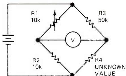
FIGURE 4. A BASIC RESISTANCE-MEASURING BRIDGE CIRCUIT.
