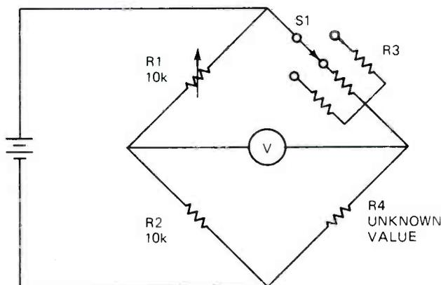
FIGURE 5. A BRIDGE CIRCUIT WITH AN EXTENDED RANGE.
