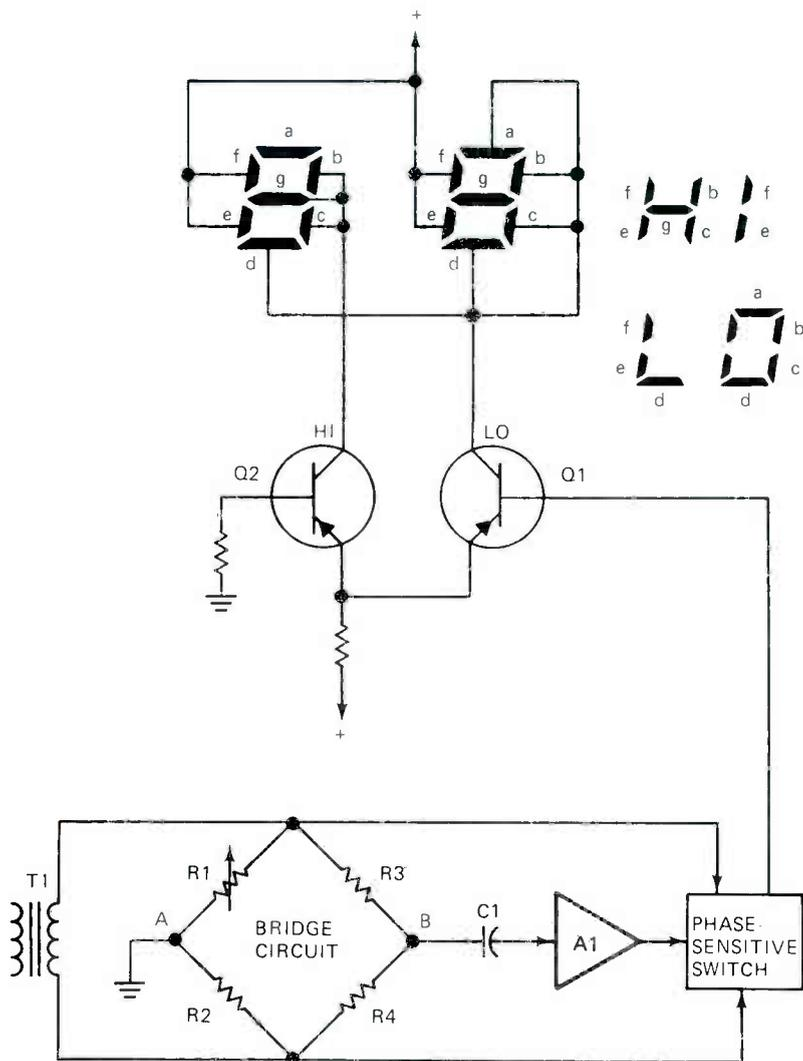
FIGURE 8. A SIMPLIFIED DIAGRAM OF THE DISPLAY CIRCUIT.
