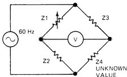
FIGURE 6. A BASIC CAPACITANCE-MEASURING BRIDGE CIRCUIT.
