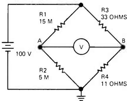
**FIGURE 3. THREE EXAMPLES OF BALANCED BRIDGE CIRCUITS.**
