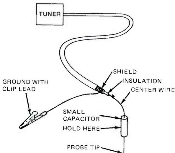
FIGURE 6. USING A TUNER AND SHIELDED COAXIAL WIRE TO INJECT A SIGNAL.
