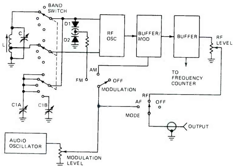
FIGURE 1. MAJOR PARTS OF THE MODEL 282 SIGNAL GENERATOR.
