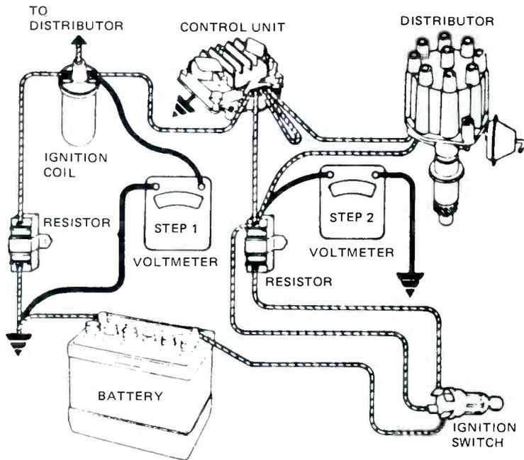
FIGURE 7. CHECKING THE PRIMARY CIRCUIT CONTINUITY WITH A VOLTMETER.
