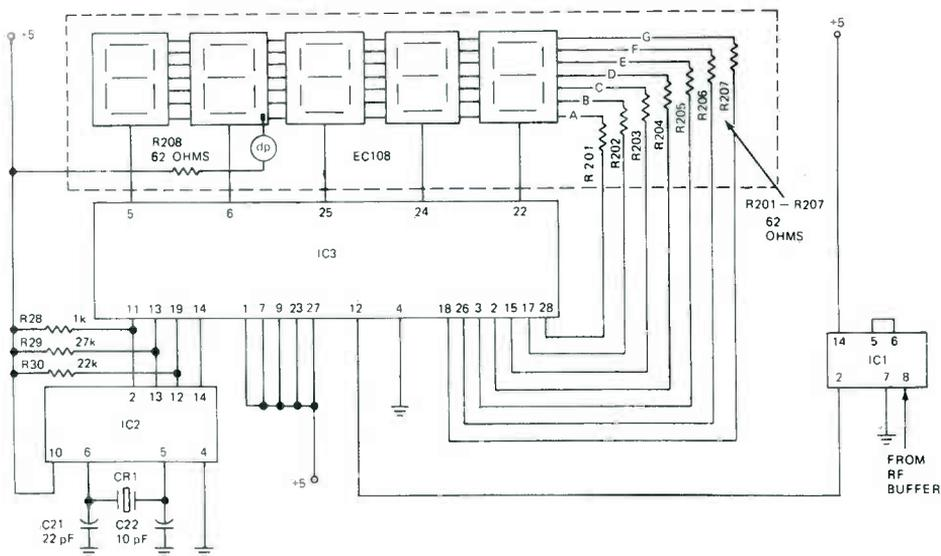
FIGURE 2. THE FREQUENCY COUNTER AND DISPLAY CIRCUIT OF THE MODEL 282.
