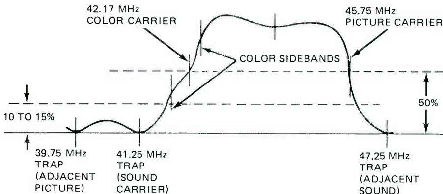
FIGURE 3. COMPLETE I-F BAND-PASS CHARACTERISTIC CURVE.
