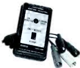
FIGURE 6. AN ELECTRONIC IGNITION ANALYZER.
