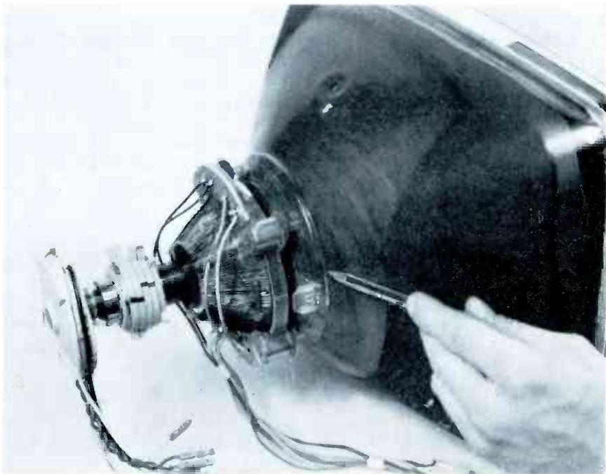
FIGURE 3. A BONDED-YOKE PICTURE TUBE. THE AREA INDICATED IS GLUED TO THE TUBE.
