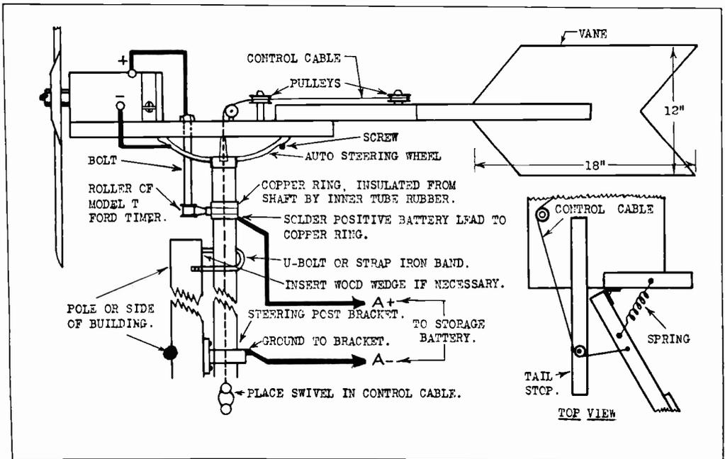
It is advisable to key the propeller to the generator shaft to prevent it from loosening and slipping on the shaft. If there is a tendency for the blade to wobble on the shaft, apply liquid solder or plastic wood to the inside of the hub.
