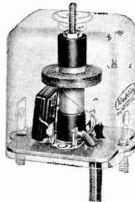
inductance of the coil which in combination with a fixed capacitor tunes to the frequency of the undesired code signals. The rejection ratio of the Polyiron wave trap is so much greater than that of the conventional air-core device that it effectively suppresses interference from code signals before it reaches the first tube of the receiver, without interfering in any way with normal reception of desired signals.
