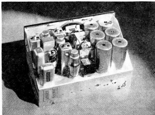
Rear view of 20A aviation receiver with cover removed.
