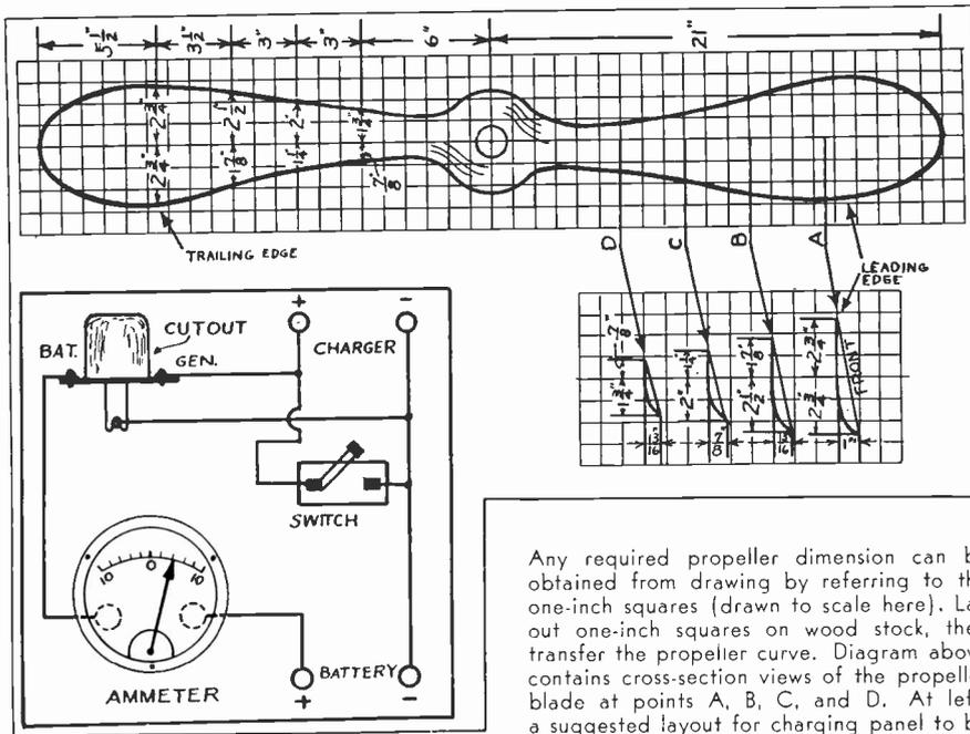
Any required propeller dimension can be obtained from drawing by referring to the one-inch squares (drawn to scale here). Lay out one-inch squares on wood stock, then transfer the propeller curve. Diagram above contains cross-section views of the propeller blade at points A, B, C, and D. At left: a suggested layout for charging panel to be located near or on the battery-charging bench.
