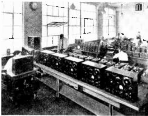
Standard signal generators and many other types of precision instruments are being calibrated and adjusted in this corner of the General Radio standardizing laboratory.
