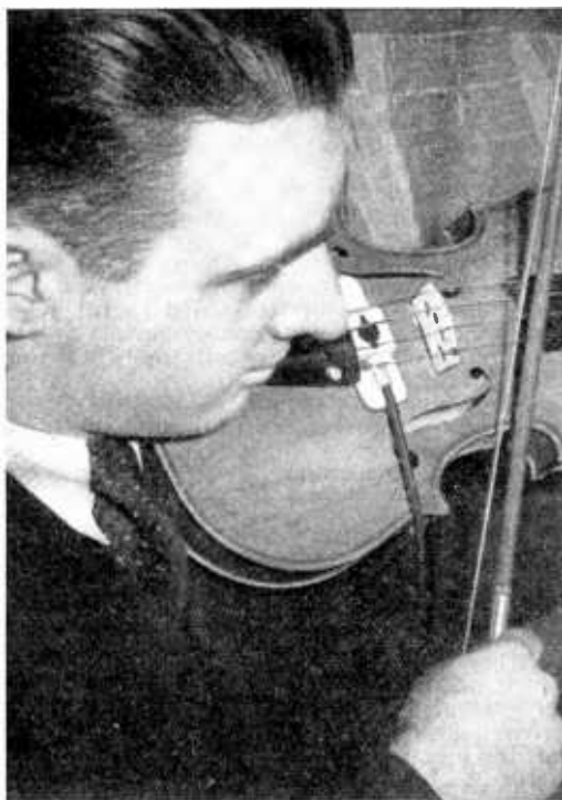
Maximilian Rex of the Ferde Grofe Orchestra uses the Amperite Kontak microphone on his violin.
