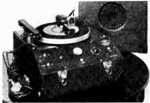
Vibro-Master model F recorder, made by Vibro-Master Successors, 2744 Broadway, New York, N. Y. Note the sound level-indicating meter in the center of the inclined panel.
