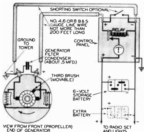
FIG. 6. Basic circuit diagram for a wind-driven battery-charging system.
