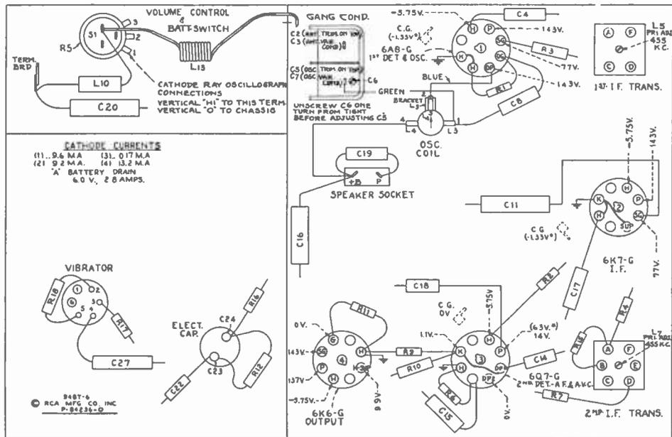
Bottom view—rear of chassis. Radiotron Socket Voltages, and Location of parts
