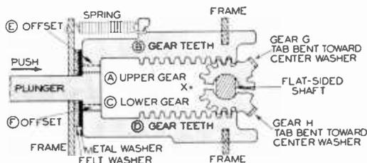
Simplified sketch of one plunger assembly in the Oak push-button tuner.
