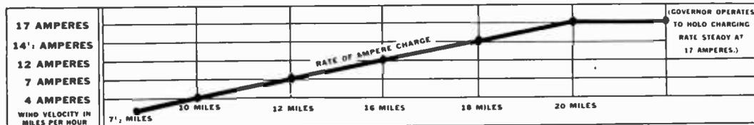
Charging rate in amperes at various wind velocities for model '39 6-volt Wincharger, made by the Wincharger Corporation, Sioux City, Iowa. Note that charging begins in this unit at a wind velocity of 7/2 miles per hour.
