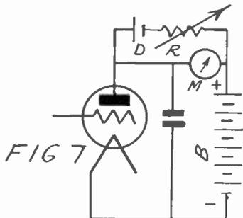
value of the A.C. input must exceed the bias enough to cause a change in the average plate current. This means that we are measuring less than the peak by some value close to .5 volt. At high voltages this is negligible, but below 10 volts, this error becomes increasingly larger. A correction chart is sometimes provided for low voltage readings.
