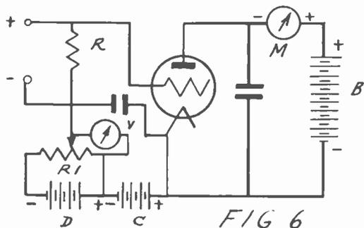
scale with no applied A.C. voltage. Then the negative voltage developed across  $R$  reduces the current, causing the meter to read in the other direction or down-scale. Thus it is calibrated in a reverse manner. The meter movement can be reversed so that maximum current causes the meter needle to move to the left, then the voltage will be indicated in the normal left-to-right manner.
