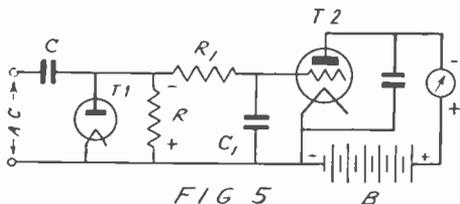
rectifier tube  $T_1$  connected across resistor  $R$  would be a large load on the source of voltage. However, the condenser  $C$  and resistor  $R$  are chosen so that the voltage developed across  $R$  is maintained as a negative voltage on the plate of the rectifier, so that current flows only at the extreme tips of the positive peaks of the applied A.C. voltage. In other words, the time constant of  $R-C$  is high, maintaining the voltage for an appreciable period of time.
