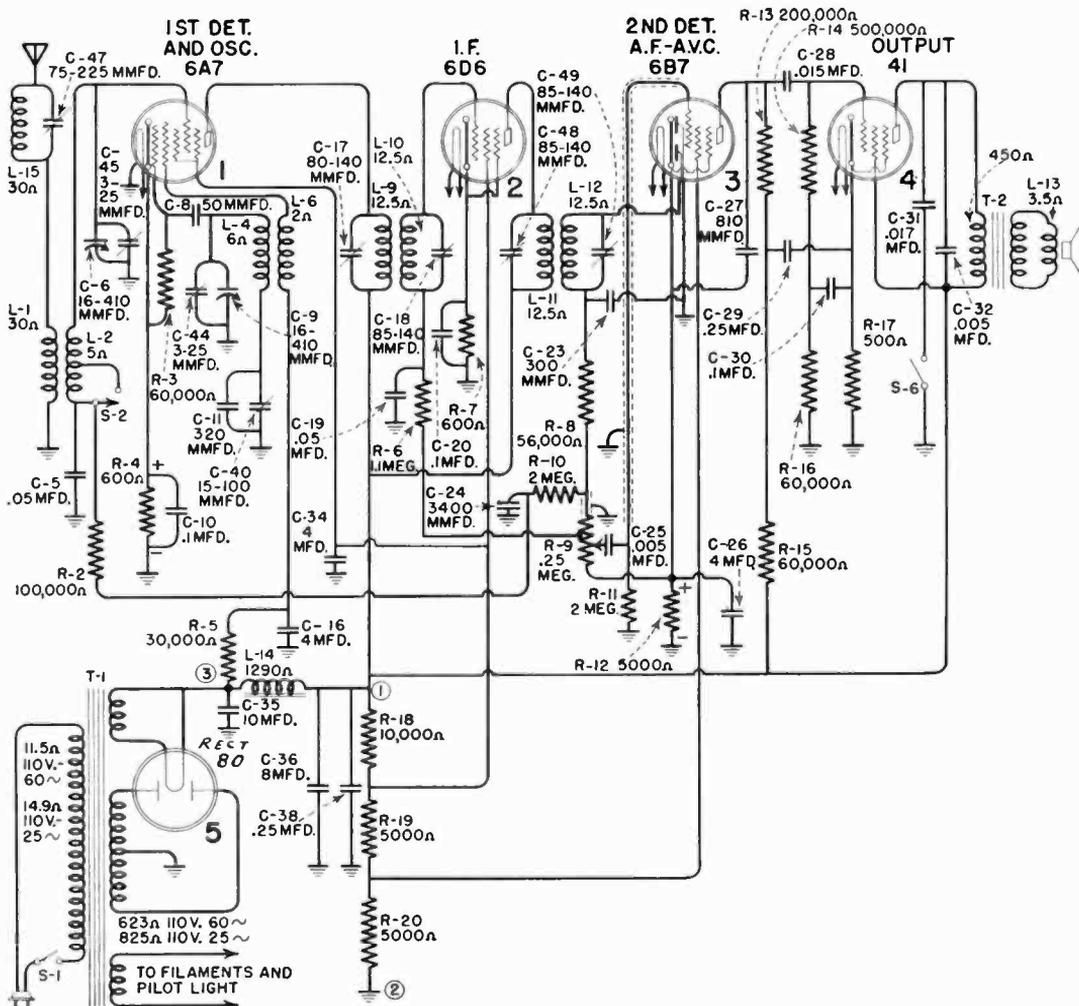
When switch S-2 is closed, the preselector is tuned to the Police Band. The second harmonic of the oscillator then beats with the Police Band stations to form the I.F. frequency.
