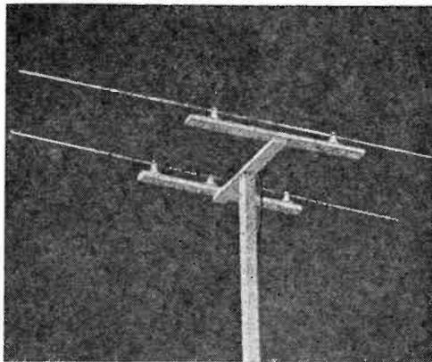
As can be seen in the drawing above, the two-element beam antenna consists of an ordinary half-wave dipole, now called the driven element, and a reflector. The latter has no connection.
