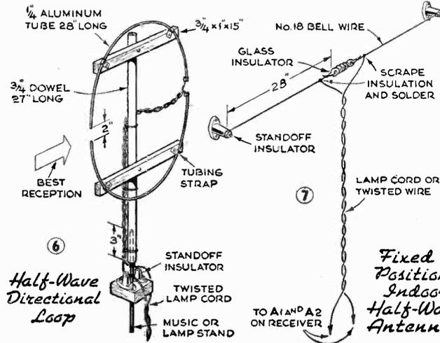
since it can readily be turned to favor any station. Drill a hole 3" in one end of the dowel, and make the diameter of the hole large enough to allow a free fit on top of a music or lamp stand. Twisted lamp-cord feeders are clamped to the ends of the aluminum semi-circles. Keep the feeder line under 12' in length.
