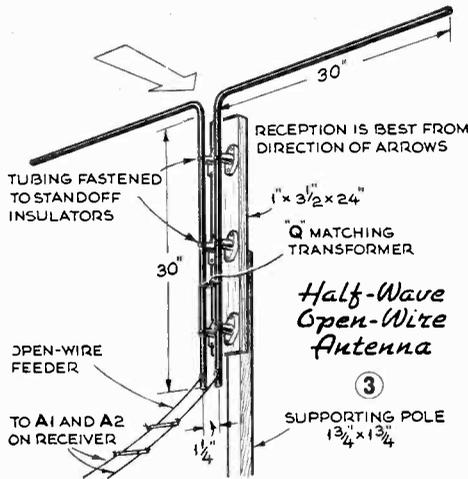
but to link it to the antenna, you will need a simple Q-matching transformer that is nothing more than two vertical legs. The combination is the half-wave antenna, open-wire line, shown in Fig. 3. Bend two aluminum tubes and bolt them to standoff insulators through 3/16" holes drilled in the tube walls. The vertical portions of the tubes must be perfectly parallel, and spaced 1 1/4" from center to center. Accuracy of the Q-matching depends on this distance.
