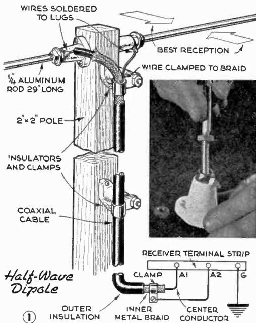
For best results the half-wave dipole should extend at least 10' above the roof of a building. Fig. 1 shows how the antenna is connected to a typical receiver terminal strip. You can use other types of low-loss feeders in place of the coaxial cable. If you do, connect one wire of the pair to each of the dipoles, and one to each of the first two terminal posts. This directional antenna favors signals coming from the directions shown by the blocked arrows.
