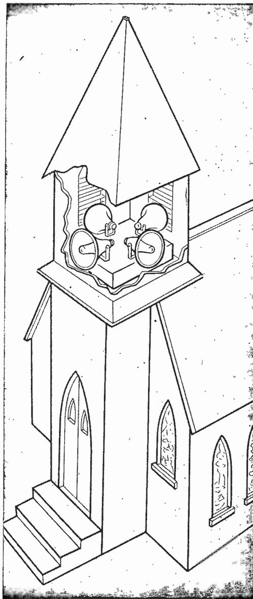
following additional refinements: microphone pickup for organ, organ chimes and choir—to be used for steeple sound distribution, indoor sound reinforcement and hard-of-hearing aids for within the church.
