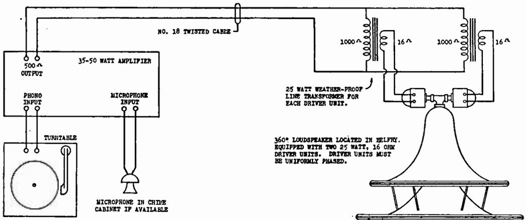
Fig. II Typical Church Steeple Installation
