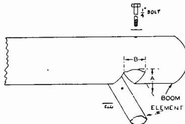
Fig. 2. The boom should be slotted so that the elements can be fastened to it with  $\frac{1}{4}$ -inch bolts.
