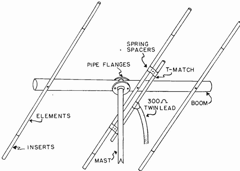
Fig. 1. The boom is made of 2-inch tubing and the elements and the T-match are made of 1-inch tubing. The inserts at the ends of the elements are made of  $\frac{7}{8}$ -inch tubing.
