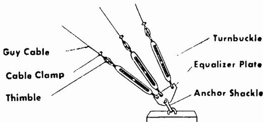
Fig. 10. Method of attaching Guy Cables to anchor support used with VEE-D-X antenna tower shown in Fig. 9.
