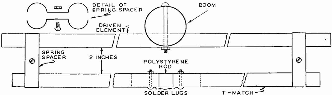
Fig. 6. The T-match is made of the same size tubing as the elements. It is spaced two inches from the driven element by means of the spacers made from 1/16-inch sheet aluminum. The transmission line is soldered to the lugs near the center of the T-Match.
