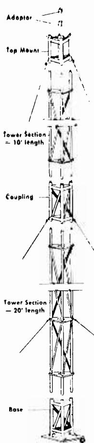
Fig. 9. Typical Antenna Tower suitable for TV antennas, manufactured by VEE-D-X.
