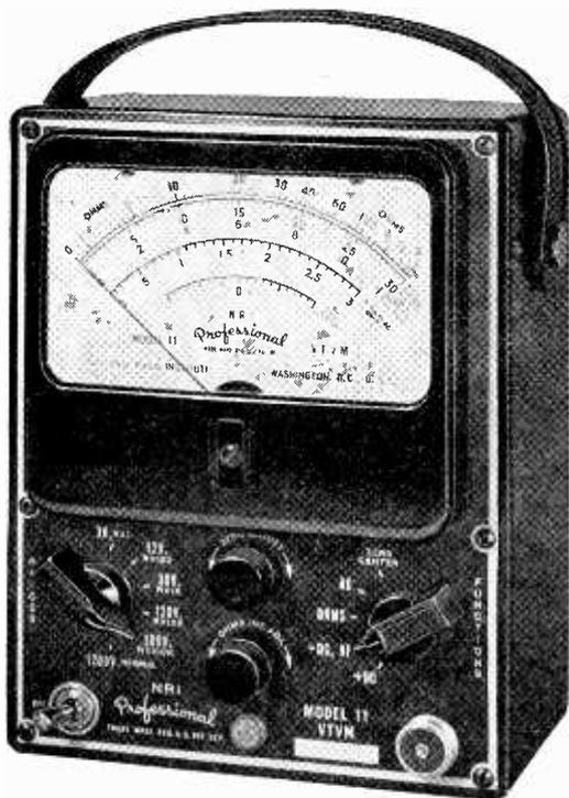
**FIG. 3. The Model 11 NRI Professional Vacuum Tube Voltmeter.**
