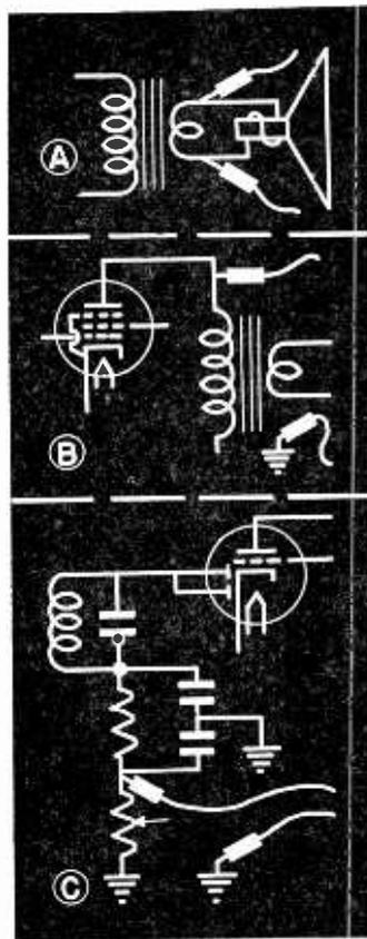
FIG. 5. Three ways of connecting a vacuum tube voltmeter for use as an output indicator in alignment: A, across the speaker voice coil; B, from the plate of the output tube to B minus; C, across the diode load. Methods A and B use the instrument as an audio voltmeter. In method C, measure the avc voltage by connecting the instrument as a dc voltmeter, with the function switch set at —DC.
