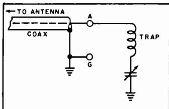
Figure 2. Series Tuned F-M Trap.
