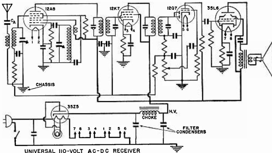
FIG. 4. Schematic of a typical AC-DC receiver.
