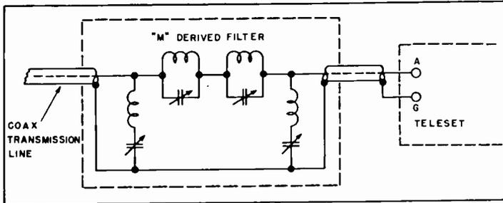
Figure 4. M Derived Band Elimination Filter.
