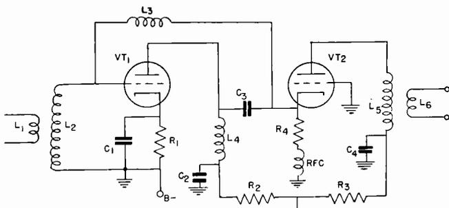
Fig. 3. The basic cascode amplifier.
