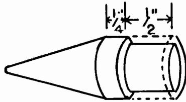
Fig. 3. Step 1—Cut one-half inch off the unshaped end of the rod and then smoothly sand it to fit into one end of the hollow tube. Care must be taken so that it is a tight fit because only pressure holds the rod in the tube. However, do not force the rod into the tube or the tube will break.
