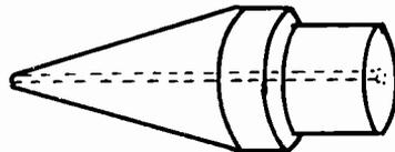
Fig. 4. Drill a hole through the center of the rod, then insert the needle. The needle must make a "snug" fit. If the drill diameter is larger than the needle diameter, then drill only part of the way; heat the needle, and force it the rest of the way.
