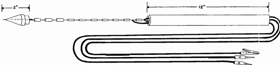
Fig. 5. This is how your finished probe will look. Slip the hollow tube down over the resistors, and fit the front end into it.
