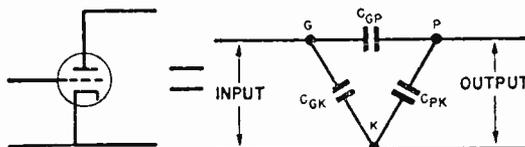
Fig. 1. The inter-electrode capacities of a triode.
