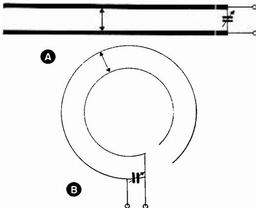
Fig. 2. (A) A quarter-wave shorted line of the type used to tune some UHF converters. (B) A line of the same type curved to form an arc.
