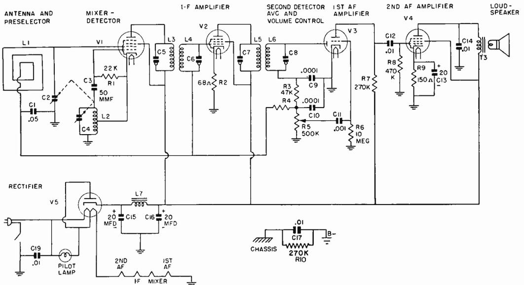
FIG. 1. Typical ac-dc receiver schematic.
