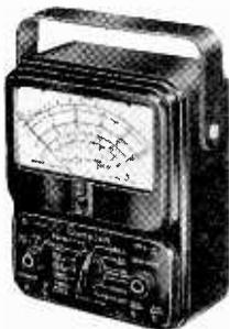
Completely portable, no AC power required. 20,000 ohms per-volt on DC, 1000 ohms per-volt on AC. Measures AC-DC volts, AC output, decibels, DC current, ohms. Size 5 1/4" x 7" x 3 1/2". Large easy-to-read, 4 1/2" meter scale. Operating instructions and tests leads included. Optional Accessories — 25,000-volt Television Probe, \$9.95. Eveready Neolite Carrying Case, \$8.75.
