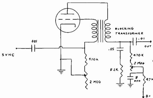
Fig. 6. Typical vertical oscillator circuit.
