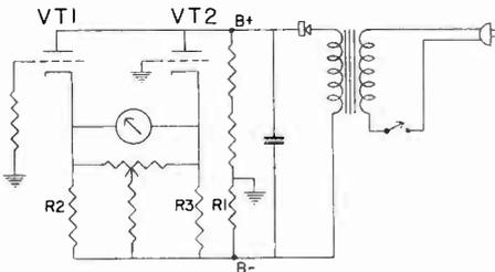
FIG. 5. The power supply circuit in the Model W VTVM.
