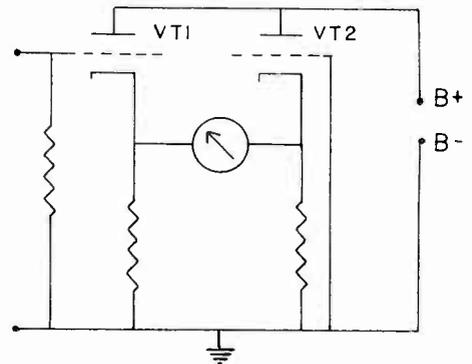
FIG. 3. The basic circuit of the VTVM. The ground connection in this and other diagrams is not a ground to chassis. It is a floating ground.
