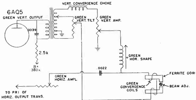
Fig. 1. Vertical and horizontal convergence adjustments for green beam.
