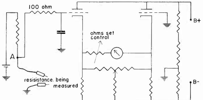
FIG. 8. The resistance measuring system.
