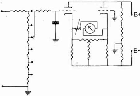
FIG. 7. The circuit change for measuring negative dc voltages.
