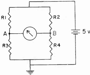
FIG. 2. A balanced bridge circuit.
