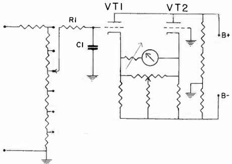
FIG. 6. The voltage divider. This permits measurements on various voltage ranges.
