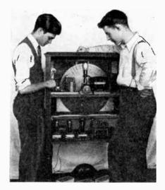
Above: View of a receiver to catch broadcast sight waves. The receiving disk, motor and neon lamp are easily recognized above. It will probably be a matter of only a short time until Television receivers will be as easily obtained as sound receivers are now.
