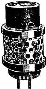
Left, Device Which Protects A. C. Tubes from Varying Line Voltage; Right, an Ingenious Assembly for Television Reception Permits Accurate Adjustment of the Neon Tube and Automatic Speed Control
