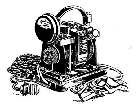
Vibrating type of retifier and stepdown transformer outfit for recharging storage batteries on the usual alterniating current supply line. The vibrating reed, which appears under the handle, rectifies both side of the alternating current so that direct current is obtained. The volume of direct current is indicated by the ammeter. Table of Contents:
