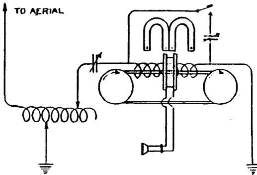
FIG. 87.—Magnetic Detector—Marconi.
