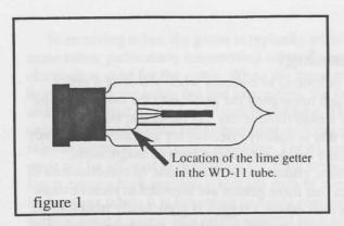
the tube. You can spot one of the lime getter tubes by looking for a white powdery deposit on the glass at the point shown in figure 1.
