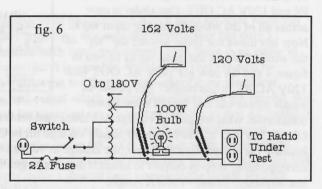
incorporating a switch from the AC plug line wouldn't be a bad idea either. If your variac isn't very big, it's probably a "control" type variac operating at a lower voltage, say 60V AC and 120V AC would pop it. But keep it anyway, we have other uses for lower voltage variacs later in this article (good junk must never be wasted!).
