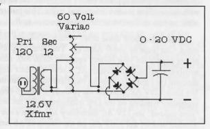
volts anyway and it is little hard to do with a tapped resistor with any accuracy. Observe figure 8a with the curcuit using a low voltage variac direct to a diode bridge and large filter capacitor. To make it a negative supply, just connect the negative to the biasing and the positive to the ground reference. One note of caution - check between your various DC circuits for AC potentials because differing designs will be fine in and of themselves for isolated DC but may short
