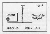
transferred, what we gain in voltage, we lose in amperes (current). That is, as OHM's law puts it; Power (watts) equals Voltage times Current (Amperes) so because the power stays the same, the change in voltage will show a corresponding drop in current to offset it in order to get the same power. Have I lost anybody? Power=Volts X Amps.
