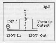
120V AC, SLOWLY. We'd start with the slider at the bottom and move it up to
